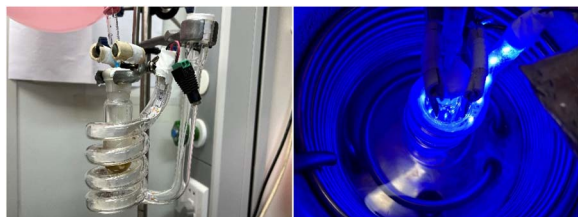
Fig. 2 The photocatalytic glycosidation apparatus designed, constructed and applied in this work.
