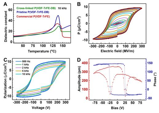
Fig. 5 Ferroelectric properties of the crosslinked P(VDF-TrFE-DB) films. (A)  $\varepsilon - T$  curves of P(VDF-TrFE) 80/20 mol%, pristine P(VDF-TrFE-DB) and crosslinked P(VDF-TrFE-DB) films at 10 kHz. (B and C) P - E loops of Au/crosslinked P(VDF-TrFE-DB)/Au under different electric fields at 1 kHz (B) and at different frequencies (C). (D) Phase–voltage hysteresis and amplitude–voltage butterfly loop from PFM measurements.
