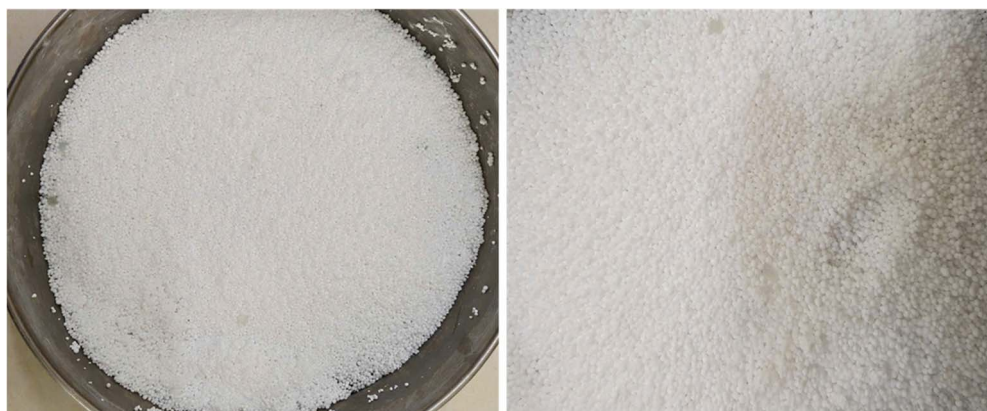
Fig. 9 Struvite pellet images from the FBHC process.
