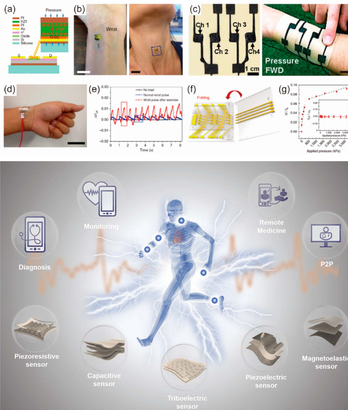
Fig. 4 Wearable pressure-sensing gadgets. (a) A schematic diagram of the cross-section of the pressure sensor and its contacts in an accompanying transistor. (b) The pressure sensor is positioned on the wrist and neck to measure instantaneous variations in blood pressure. Produced with copyright permission from MDPI, Polymer. 69 (c) A printed pressure sensor is mounted on a commercially available elastomeric patch. (d) The skin-mounted sensor is positioned directly above the wrist artery (at a scale bar of 3 cm). (e) The heartbeat is measured by sensing the physical force under healthy and exercising conditions. (f) A representative picture of pressure-sensitive graphene FETs (g). A plot of changes in normalized drain current versus pressure applied to the device. Wearable pressure sensors for monitoring human health. By integrating biomechanical devices with artificial intelligence, including active materials, functional structures, wireless transmission technology, and big data analysis, convenient and biocompatible assessment of the cardiovascular system can be achieved. Such an intelligent platform provides personalized healthcare and therapy to individuals while maintaining user comfort, superior sensitivity, long life, ease of use, and mechanical durability. Reproduced from ref. 31 and 74. With permission from [Royal Society of Chemistry], copyright [2023] & Wiley 2022.
