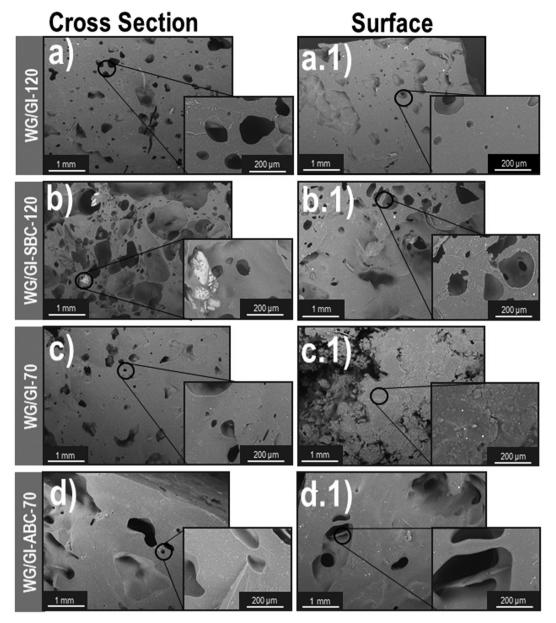
Fig. 3 Microstructure of the WG pad layers: The column (a-d) shows the cross-sections, and the column (a.1-d.1) shows the surface structure.
