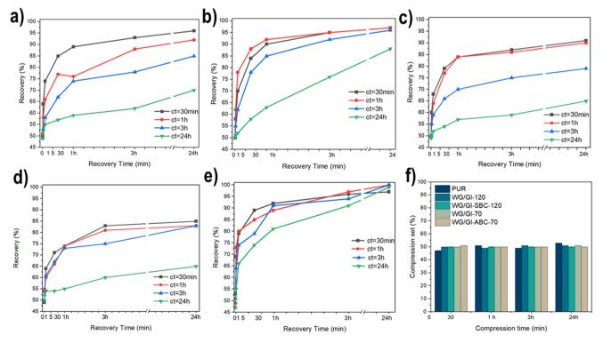
Fig. 6 Recovery of the samples as a function of recovery time after different periods of compression time: (a) WG/Gl-120, (b) WG/Gl-SBC-120, (c) WG/Gl-70, (d) WG/Gl-ABC-70, (e) PUR. (f) Compression set values directly after stress release (ca. 1 s). Note: the values are not significantly different (P < 0.05).
