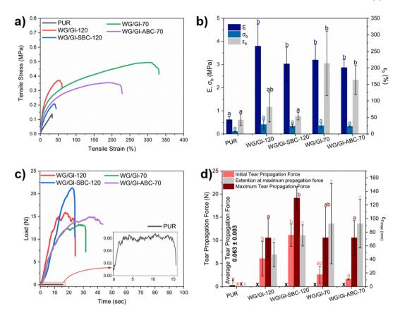
Fig. 7 (a) Tensile stress-strain curves of the WG pad and PUR layers and (b) average E (Young's Modulus), tensile stress at break (σ<sub>b</sub>) and tensile elongation at break (En). (c) Load-time charts for WG-based layers (highly extensible) and PUR (low extensible) and (d) average tear propagation force and maximum extension before total fracture. Note: the values (within the same color group) are not significantly different (P < 0.05).
