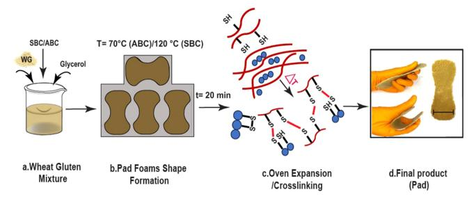
Fig. 1 Experimental protocol for the production of the protein pad layers, involving the mixing of the protein, glycerol and foaming agent (a), spreading the mixture in the moulds evenly for the oven expansion process (b), allowing for the formation of crosslinks between glutenin (represented by red chains containing -SH) and gliadin (represented by blue units containing -S-S-) in the protein matrix and foaming induced by the bicarbonates (c). The scale bar in the final pad (d) is 5 cm.
