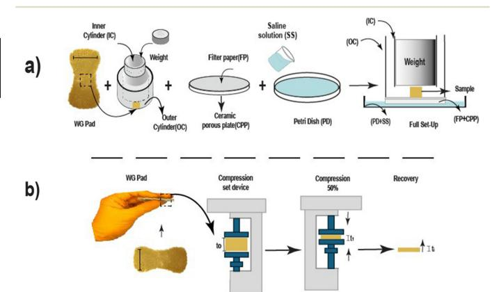
Fig. 2 Schematic illustration of (a) the Absorbance Under Load (AUL) set-up and (b) the Compression Set test. The scale bar in the WG pad layer is 5 cm.
