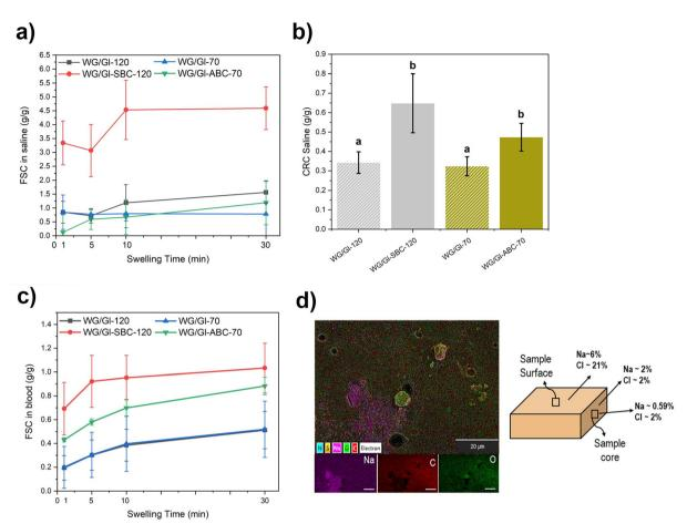
Fig. 4 Free swelling capacity in saline (FSC, a) and the centrifugation retention capacity after 30 min of saline swelling (CRC, b). (c) Free swelling capacity in defibrinated sheep blood. (d) Elemental analysis by EDS of the WG/GI-SBC-120 cross-section. The scale bars in the inserts of d are 20  $\mu$ m. Note: different letters mean the values are significantly different (P < 0.05).
