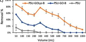
Fig. 5 a) Experimental setup used for the adsorption test of CBZ and the removal performance of b) PSU, PSU-GO-A and PSU-GOLys-A and c) PSU, PSU-GO-B and PSU-GOLys-B.
