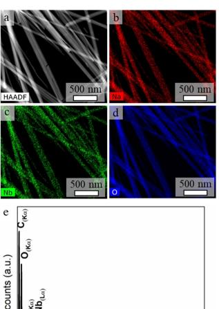
10 12 14 16 6 18 energy (KeV) Fig. 4 (a) High-angle annular dark-field (HAADF) scanning TEM (STEM) image of SOMS-based nanorods and corresponding elemental maps obtained by energy dispersed X-ray spectroscopy (EDS) for (b) Na, (c) Nb, and (d) O. (e) An EDS spectrum corresponding to the average composition of the nanorods, which further confirms the presence of Na, Nb, and O in the product. The source of the Cu signals in the spectrum was the TEM grid supporting the sample
