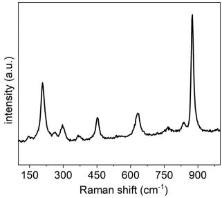
Fig. 5 Room temperature Raman spectrum for the SOMS-based nanorods obtained using an excitation at 514 nm and a scan rate of 10 cm<sup>-1</sup> per second.
