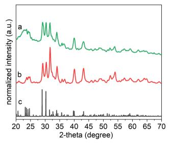
Fig. 7 (a) Powder XRD patterns of SOMS after exposure to 14.1 MeV neutrons for 72 h. For comparison, powder XRD patterns are also included for (b) pristine SOMS before exposure to neutrons, and (c) a reported SOMS reference sample (ICSD No. 55415).
