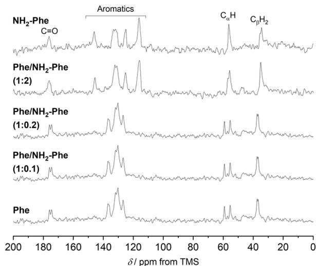
Fig. 9  $^1\text{H}$ - $^{13}\text{C}$  CP/MAS NMR spectra of Phe (303 mM), Phe/ $\text{NH}_2$ -Phe (1 : 0.1), Phe/ $\text{NH}_2$ -Phe (1 : 0.2), Phe/ $\text{NH}_2$ -Phe (1 : 2) and  $\text{NH}_2$ -Phe (606 mM) hydrogels acquired with an MAS rate of 8.5 kHz using a 400 MHz solid-state NMR spectrometer.
