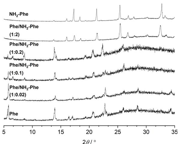
Fig. 8 PXRD patterns of Phe (303 mM), Phe/ $\text{NH}_2$ -Phe (1 : 0.02), Phe/ $\text{NH}_2$ -Phe (1 : 0.1), Phe/ $\text{NH}_2$ -Phe (1 : 0.2), Phe/ $\text{NH}_2$ -Phe (1 : 2) and  $\text{NH}_2$ -Phe (606 mM) hydrogels.
