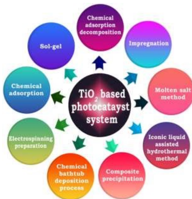
Figure 16. Schematic representation of various synthesis strategies of TiO 2 -based photocatalyst system reported in the literature.
