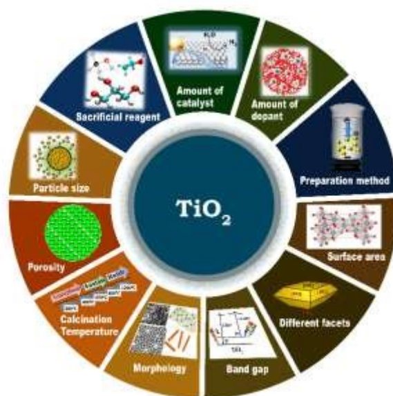
Figure 15. Schematic representation of the various factors which determine the photocatalytic hydrogen evolution activity of TiO 2 -based photocatalysts.
