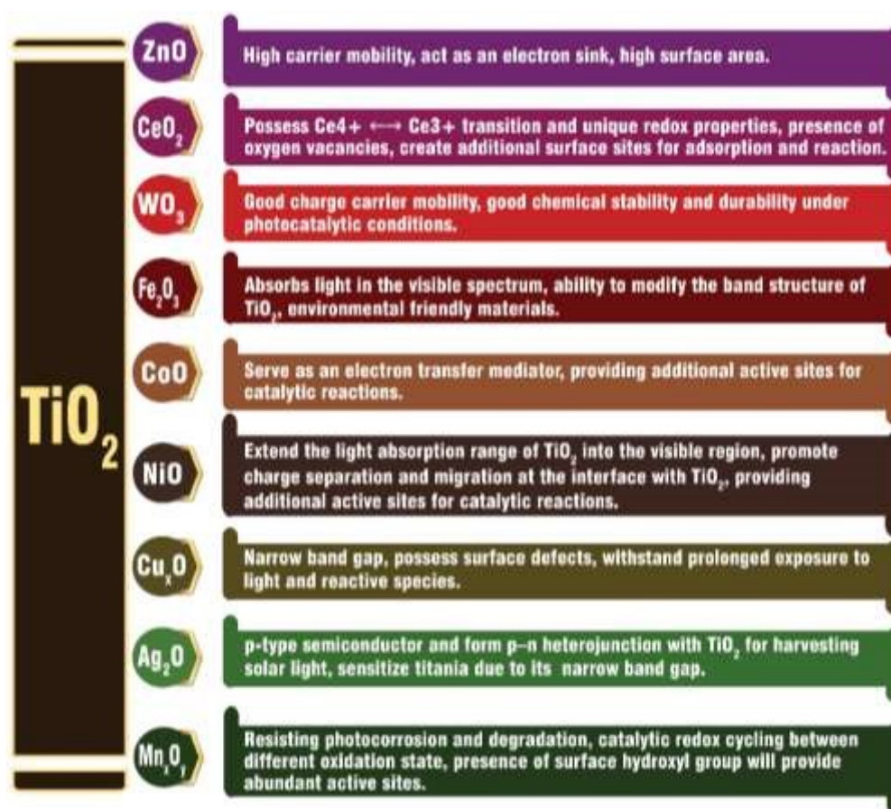
Figure 9. Schematic representation of various metal oxides used for improving the photocatalytic hydrogen evolution activity of TiO 2 .
