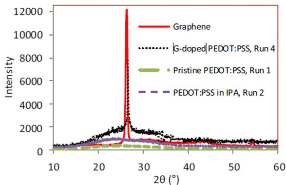
Fig. 10 XRD patterns of graphene, pristine PEDOT:PSS thin film (run 1), PEDOT:PSS thin film prepared using IPA as a co-solvent (run 2), and SVAC-fabricated graphene-doped PEDOT:PSS (run 4).<sup>180</sup>
