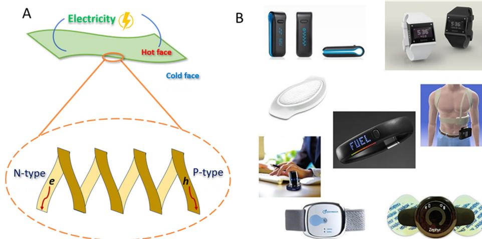
**Fig. 2** (A) A flexible OTE device is depicted, consisting of alternating p-type and n-type semiconducting materials. The device can be made using wearable functional fabric that converts waste body heat into electricity through high energy transfer from a hot face to a cold face. (B) Potential use of organic thermoelectric generators (TEGs) is demonstrated, supporting wearable electronics, such as watches, fitness trackers, health monitoring devices, and toys.
