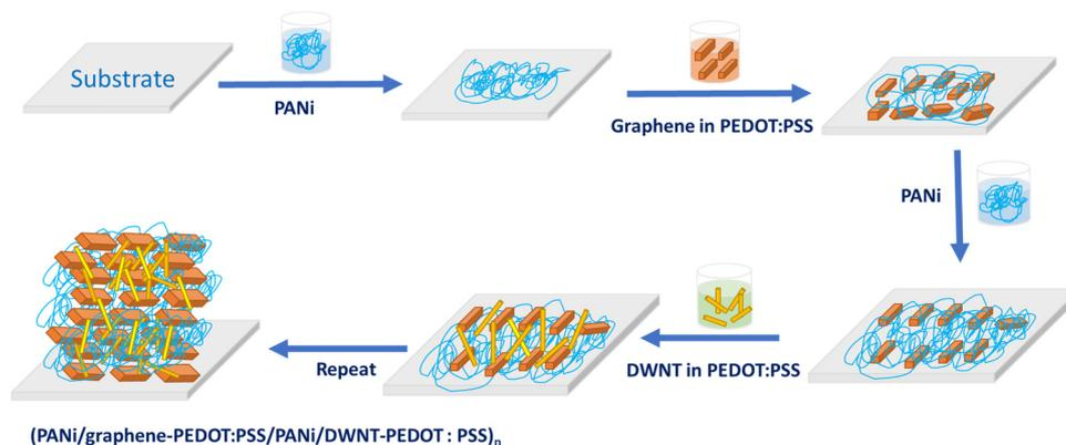
Fig. 7 Layer-by-layer deposition method of PANi/graphene-PEDOT:PSS/PANi/DWNTs-PEDOT:PSS hybrids.
