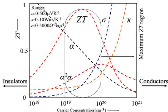
Fig. 5 Thermoelectric parameters with variations in carrier concentration taken from ref. 50, where  $\alpha$  represents the Seebeck coefficient,  $\sigma$  represents the electrical conductivity,  $k$  represents the thermal conductivity, and  $ZT$  represents the figure of merit. The image was adapted with permission from Prasad *et al.*,<sup>51</sup> Springer Nature 2020.
