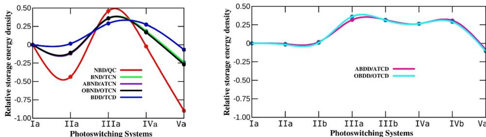
Fig. 3 Variation in the energy storage density of *N*-substituted systems relative to that of their parent photoswitching system. The energy values were obtained by computing the electronic energy with the DLPNO-CCSD(T)/Def2TZVP method and including thermal correction at the M062X/6-311++G\*\* level.
