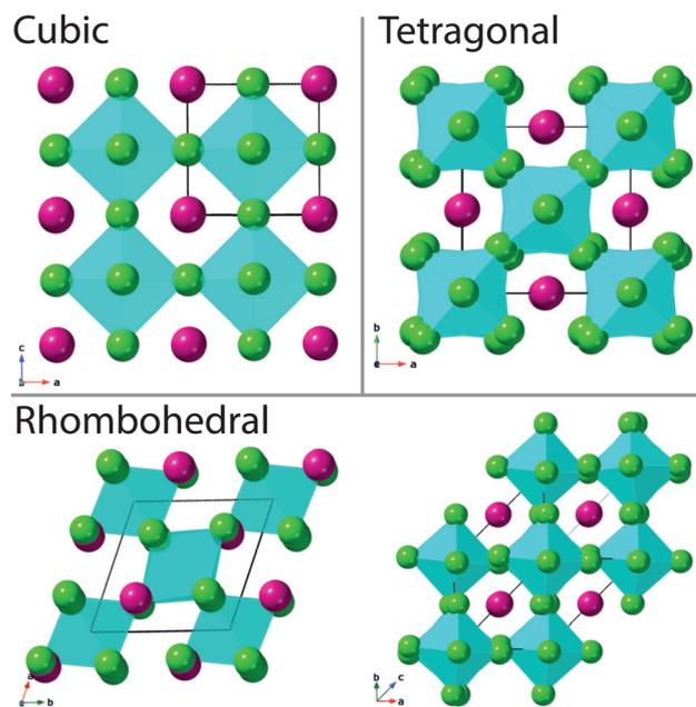
Fig. 1 Crystal structure of cubic aristotype perovskite, ABX<sub>3</sub>, and the tetragonally and rhombohedrally distorted variants. In all three structures the A-site atoms are shown in purple, the X-site atoms are green and the B-site atoms are within the green BX<sub>6</sub> octahedra. The solid black lines outline the crystallographic unit-cell in each structure.
