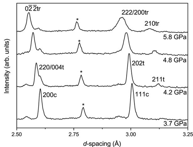
Fig. 6 Changes in diffraction pattern of CsCaCl<sub>3</sub> with increasing pressure across the phase transition region. In the bottom trace the reflections from the cubic (c) phase are identified and those from lead identified by an asterisk. Upon increasing pressure the  $R$  point reflection from the tetragonal (t) phase appears (211t) and other reflections are split. At higher pressure the splitting which occurs from the rhombohedral (tr) phase is observed.
