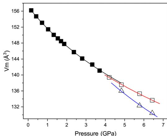
Fig. 7 Variation in unit-cell volume per formula unit ( $V_m$ ) with pressure of  $\text{CsCaCl}_3$ . The filled square for the cubic phase, unfilled red squares the tetragonal phase and the unfilled blue triangles the rhombohedral phase. The solid lines are the fitted Birch–Murnaghan EoS to the data points as described elsewhere. The number of formula units per unit cell ( $Z$ ) of the cubic phase is 1, 4 for the tetragonal phase and 2 for the rhombohedral phase.
