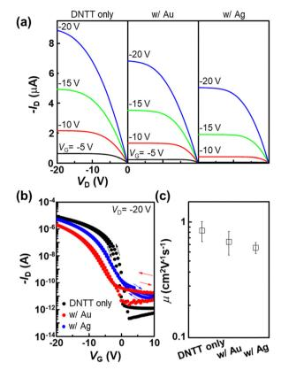
Fig. 2 Electrical characterization of DNTT OFETs incorporated with metal NPs. (a) Transistor output characteristics and (b) dual-sweep transfer curves measured in the saturation regime of DNTT OFETs without/with Au or Ag NPs. (c) Field-effect mobilities extracted from OFETs.
