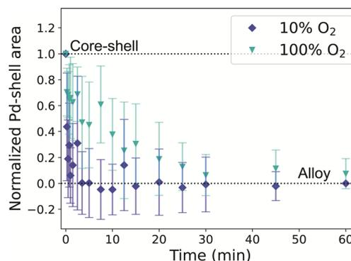
Fig. 5 *In situ* STEM visualizing the alloying of Au-Pd core-shell NPs in  $O_2$  at 375 °C. The plot shows the normalized Pd-shell area as a function of time for a 10%  $O_2$  in Ar (dark blue) and 100%  $O_2$  (light blue) gas atmosphere. The error bars represent the standard deviation of the Pd shell related area across measurements in multiple nanoparticles.
