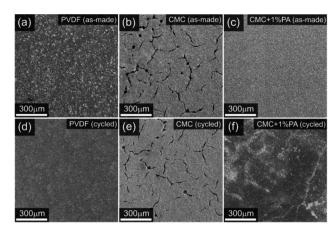
Fig. 6 Secondary electron images of electrodes before and after cycling with different binders. (a) and (d) PVDF, (b) and (e) CMC and (c) and (f) CMC + 1% of phosphoric acid (PA). Reprinted with permission of ref. 142, Copyright 2023, RSC.
