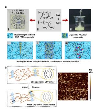
Fig. 12 (a) Rigid self-healing PAA-PAH copolymers repaired using the intermediary healing agent with the same composition under ambient conditions. Copyright 2023, Chinese Chemical Society. Reproduced with permission from ref. 115. (b) The phase-separated nanostructures of the PI-PUU copolymer. Copyright 2021, American Chemical Society. Reproduced with permission from ref. 15.
