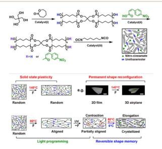
Fig. 13 A single-component robot using a programmable semicrystalline SMP with thermo-and photo-reversible bonds. Copyright 2018, AAAS. Reproduced with permission from ref. 124.
