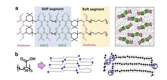
Fig. 2 (a) Typical nanostructure of synthetic poly(urethane-urea) composed of stiff and soft segments. Copyright 2021, Wiley-VCH. Reproduced with permission from ref. 22. (b) Polyethylene brush polymer with precise hairpin architecture. Copyright 2017, American Chemical Society. Reproduced with permission from ref. 32.
