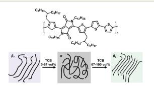
Fig. 4 The gradual  $\beta_1$ - $\alpha$ - $\beta_2$  phase transition of D-PDPP4T-HD by adding TC into CF from 0 vol% to 100 vol%. Copyright 2019, Springer Nature. Reproduced with permission from ref. 43.
