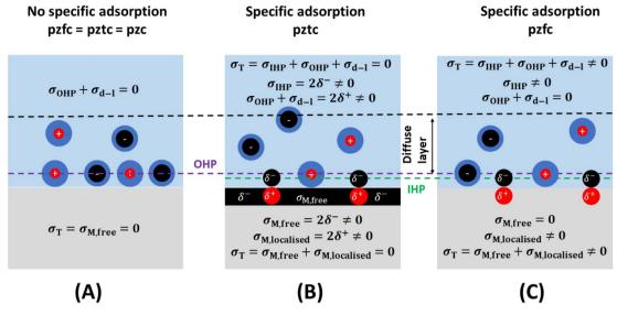
Fig. 3 The pzfc and the pztc. In the absence of specific adsorption (A), the pztc and the pzfc coincide. When there are specifically adsorbed species on the metal surface (B and C), the free charge density on the metal surface is not zero at the pztc (B), while the total charge density is not zero at the pzfc (C).
