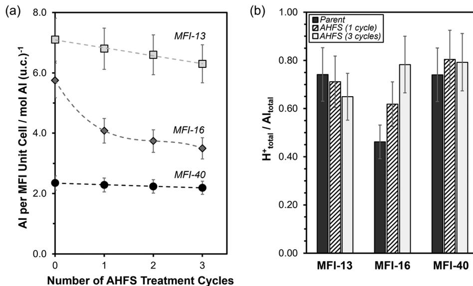
**Fig. 2** (a) Total Al content per MFI unit cell (96 T atoms) and (b) bulk  $H^+_{\text{tot}}/Al_{\text{tot}}$  molar ratio as a function of the number of AHFS-treatment cycles. Dashed lines in (a) serve to guide the eye. Error bars in (a) reflect uncertainties ( $\pm 10\%$  in (a) and  $\pm 15\%$  in (b)).
