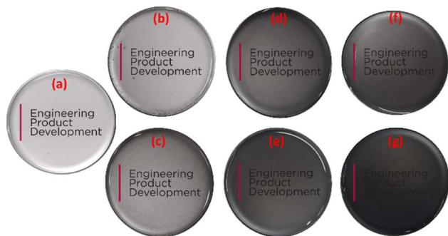
Fig. 1 Photographic images of the fabricated test structures: (a) neat PDMS, (b) PDMS–SWCNT (sily, 0.05 wt%), (c) PDMS–SWCNT (COOH, 0.05 wt%), (d) PDMS–SWCNT (sily, 0.5 wt%), (e) PDMS–SWCNT (COOH, 0.5 wt%), (f) PDMS–SWCNT (sily, 1 wt%), (g) PDMS–SWCNT (COOH, 1 wt%).
