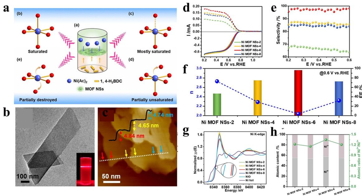
**Fig. 2** (a) Illustration of the synthetic method for Ni MOF NSs. (b) TEM and (c) AFM images of Ni-MOF NS-6. (d) LSV curves and (e) H<sub>2</sub>O<sub>2</sub> selectivity. (f) The number of electrons transferred ( $n$ ) and the Faraday efficiency. (g) XANES spectra for Ni MOF NS-2, 4, 6, 8, NiO and Ni foil. (h) The atomic content of Ni<sup>2+</sup> and Ni<sup>3+</sup>, and the atomic ratio of Ni<sup>2+</sup>/Ni<sup>3+</sup> in Ni MOF NS-2, 4, 6 and 8. Copyright 2021, WILEY-VCH.
