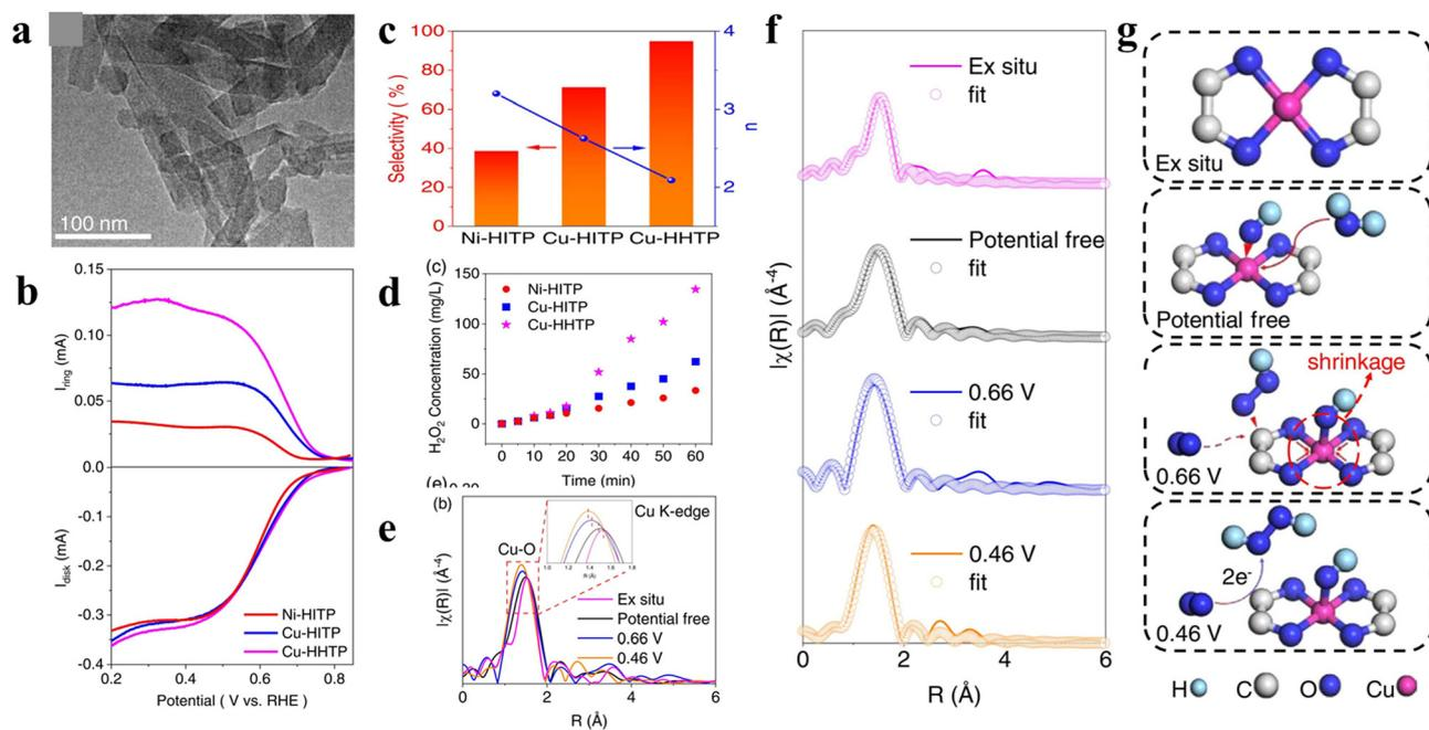
Fig. 3 (a) TEM image of Cu-HHTP. (b) LSV curves. (c)  $\text{H}_2\text{O}_2$  selectivity and the electron transfer number of Ni-HTP, Cu-HTP and Cu-HHTP. (d) Cumulative  $\text{H}_2\text{O}_2$  yield. (e) FT-XAFS curves for Cu-HHTP. (f) The FT-XAFS fitting results of Cu-HHTP. (g) Scheme of the proposed 2e ORR mechanism for Cu-HHTP. Copyright 2022, Elsevier.
