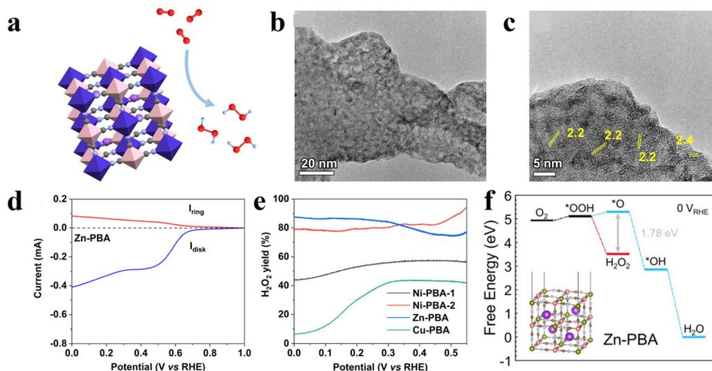
**Fig. 1** (a) Illustration of the M-PBA structure. (b) and (c) TEM images of the Zn-PBA catalysts. (d) LSV curves, (e) selectivity of Zn-PBA, and (f) free-energy diagrams for the ORR on Zn-PBA. Copyright 2022, American Chemical Society.
