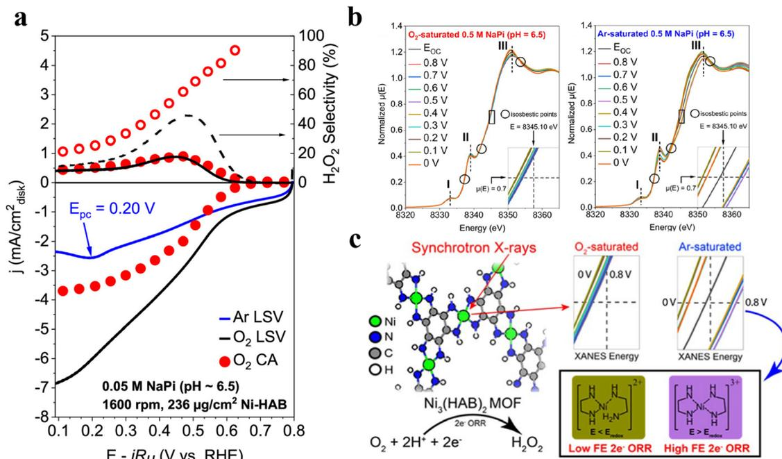
Fig. 4 (a) LSV curves of Ni-HAB. (b) XANES spectra of Ni-HAB/CFP at various applied potentials in O<sub>2</sub> saturated and Ar saturated electrolytes. (c) Schematic illustrating the changes in the nickel oxidation state during the 2e<sup>-</sup>ORR process. Copyright 2022, American Chemical Society.
