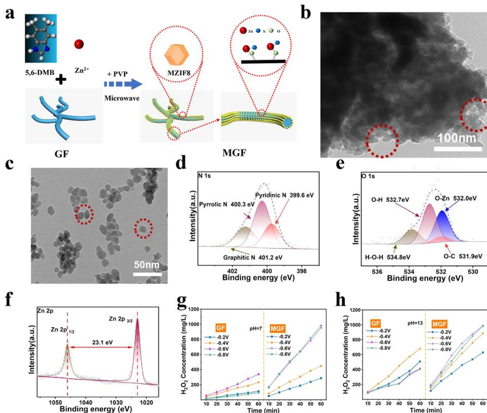
**Fig. 8** (a) Schematic showing the synthesis process of MGF. TEM images of (b) MGF and (c) MZIF8. High-resolution XPS spectra of (d) N 1s, (e) O 1s and (f) Zn 2p for MGF. (g)  $\text{H}_2\text{O}_2$  concentration over the reaction time at various solutions of MGF and GF: (g) pH = 7 (0.5 M  $\text{Na}_2\text{SO}_4$ ), and (h) pH = 13 (0.1 M KOH). Copyright 2023, American Chemical Society.
