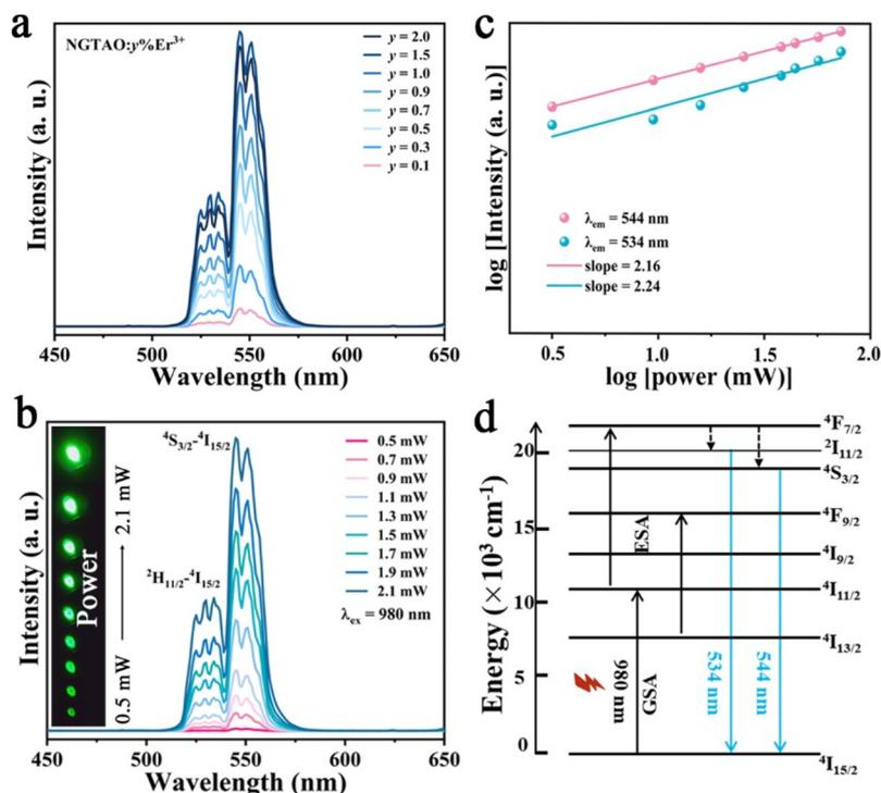
**Fig. 4** Dependence of the UCL spectra on the 980 nm laser power density. (a) PL spectra of NGTAO:y%Er<sup>3+</sup> (0.1 ≤ y ≤ 2.0) under 379 nm excitation. (b) UCL spectra of NGTAO:1.0%Er<sup>3+</sup> at different pump powers and (c) double logarithmic plots of excitation power versus UCL intensity of Er<sup>3+</sup> at 534 nm and 544 nm for NGTAO:1.0%Er<sup>3+</sup>. (d) Energy level diagram and corresponding possible UC processes of NGTAO:Er<sup>3+</sup>.
