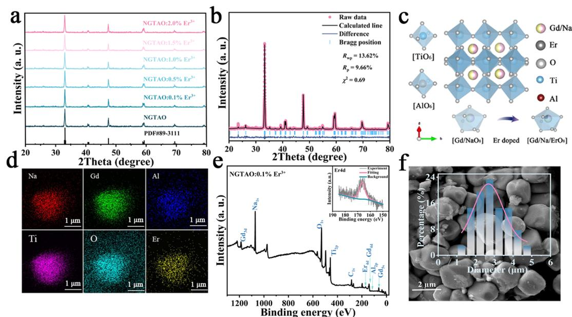
**Fig. 1** Morphological and structural characterization: (a) XRD patterns with different  $\text{Er}^{3+}$  concentrations. (b) Rietveld refinement of the powder XRD profile. Inset: calculated parameters. (c) The crystal structure of NGTAO. (d) The mapping images of the elements Na, Gd, Al, Ti, and O, respectively. (e) The XPS survey spectrum of NGTAO:0.1%  $\text{Er}^{3+}$ . Inset: XPS spectrum of Er 4d. (f) SEM of NGTAO: $y\text{Er}^{3+}$ .
