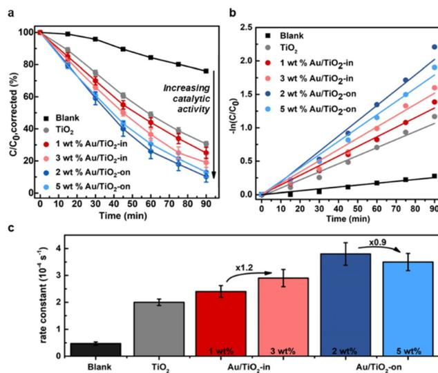
**Fig. 4** Photocatalytic degradation of 15 μM MB under light illumination (200–2500 nm). (a) Fraction of MB concentration remaining in the reaction solution ( $C/C_0$ ) as a function of time. (b) MB decomposition kinetics expressed as  $-\ln(C/C_0)$  over reaction time, and (c) the correspondingly derived first-order rate constants.
