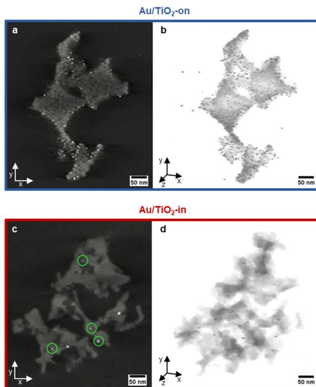
**Fig. 3** 3D analysis of the NP placement using electron tomography. XY-slices taken from the 3D reconstruction showing the interior of the 5 wt% (a) Au/TiO<sub>2</sub>-on and 3 wt% (c) Au/TiO<sub>2</sub>-in IO films and the corresponding 3D XYZ views in (b and d). Au NPs are shown as bright white spots in (a and c) and dark spots in (b and d). The green circles in (c) indicate embedded Au NPs.
