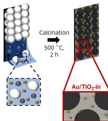
**Fig. 1** Schematic illustration of Au/TiO<sub>2</sub> IO film synthesis in which Au NPs are placed either (a) on the TiO<sub>2</sub> surface via a two-component co-assembly approach, or (b) in the TiO<sub>2</sub> matrix via a three-component co-assembly approach.
