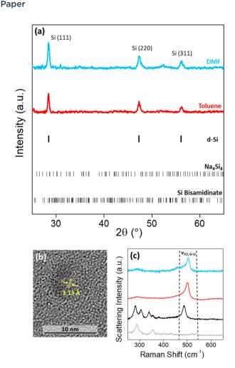
Fig. 3 (a) Powder XRD patterns of product produced in (blue) DMF and (red) toluene with Bragg peak positions plotted for diamond cubic Si,  $Na_4Si_4$  and silicon bisamidinate precursors. (b) HRTEM image of an individual particle produced in DMF showing lattice fringes corresponding to d-spacing of (111) cubic Si plane. (c) Raman spectra of (black) silicon bisamidinate, (grey) sodium silicide, and particles produced in (blue) DMF and (red) toluene.
