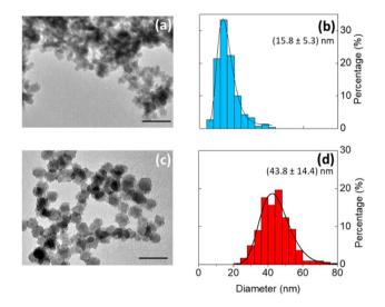
Fig. 4 (a and c) Bright field TEM images, and (b and d) particle size distribution of silicon particles produced in (a and b) DMF and (c and d) toluene. Scale bars represent 100 nm. All particle sizes were determined by analysis of TEM images (300 particles counted), sizes are given as  $(\bar{x} \pm \sigma_x)$  nm and fitted using a log-normal distribution.
