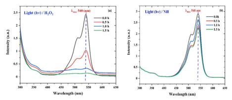
Fig. 15 (a) The UV absorption degradation curves of RhB dye with Zn-AC catalyst suspension system for the hydrogen peroxide ( $H_2O_2$ ) experiment in the presence of light ( $h\nu$ ). (b) The UV absorption degradation curve of RhB dye with Zn-AC catalyst suspension system for hydrogen peroxide ( $H_2O_2$ ) control experiment (without  $H_2O_2$  in the presence of light ( $h\nu$ ).
