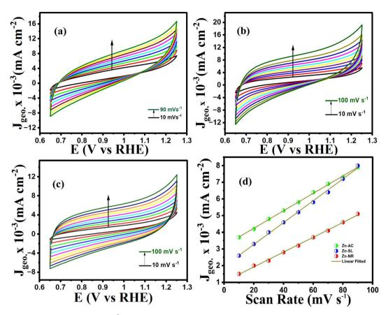
Fig. 14 Cyclic voltammograms (10–100 mV s<sup>-1</sup> capacitive region) of (a) Zn-AC, (b) Zn-SL, and (c) Zn-NR catalysts. (d) J vs. scan rate for the calculation of  $C_{\rm dl}$  (proportional to ECSA) values.
