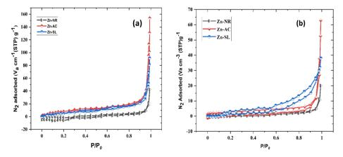
Fig. 16 (a)  $N_2$  adsorption—desorption isotherm of the three catalysts used (Zn-AC, Zn-SL, and Zn-NR), indicating the changes in the surface area of the catalysts (pre- and post-use) by Brunauer–Emmett–Teller (BET) analysis (before use) and (b) isotherm curves after the use of the catalysts.
