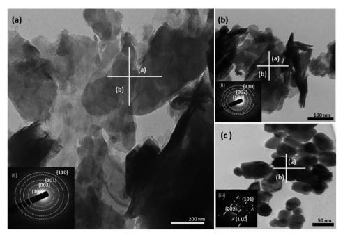
Fig. 7 The TEM (a-c) images of the three structurally different ZnO NPs from different salt precursors, i.e., sheet-like structure from zinc nitrate (a), zinc sulphate (b), and sphere-like structure from zinc acetate (c). The corresponding SAED pattern (inset figure) for the three samples shows the polycrystallinity of the samples (a and b), while the SAED pattern for sample (c) shows a shift toward a monocrystalline material.
