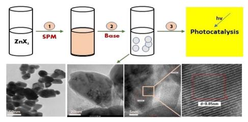
Fig. 1 A schematic diagram representing the green synthesis of ZnO NPs and their photocatalytic application
