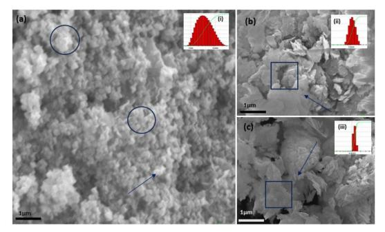
Fig. 5 The SEM (a-c) images of the three structurally different ZnO NPs from three different salt precursors, i.e., sphere-like structure from zinc acetate (a) and sheet-like structure from zinc nitrate (b) and zinc sulphate (c). DLS analysis for three samples with varying (but narrow size distribution) PDI of 0.486 for acetate (a), 0.222 for nitrate (b), and 0.277 for sulphate (c) in the top inset figure.
