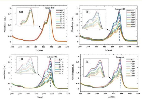
Fig. 10 UV-visible absorption spectrum of a rhodamine dye (conc.  $0.596 \times 10^{-3}$ ) and photocatalyst (conc. 100 mg L<sup>-1</sup>) suspension system under exposure to direct sunlight recorded at the time interval of 0.5 h. (a) The control experiment (dye-catalyst system in the dark) and (b) Zn-SL, (c) Zn-AC and (d) Zn-NR catalyst systems.
