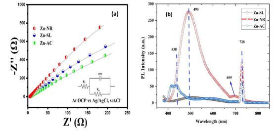
Fig. 13 (a) The electrochemical impedance spectra of the Zn-AC, Zn-SL, and Zn-NR catalysts showing different charge transfer resistance ( $R_{ct}$ ) at the electrode/electrolyte interface. (b) The photoluminescence spectra of the same catalysts showing their (e<sup>-</sup>) and (h<sup>+</sup>) pair recombination behaviour.
