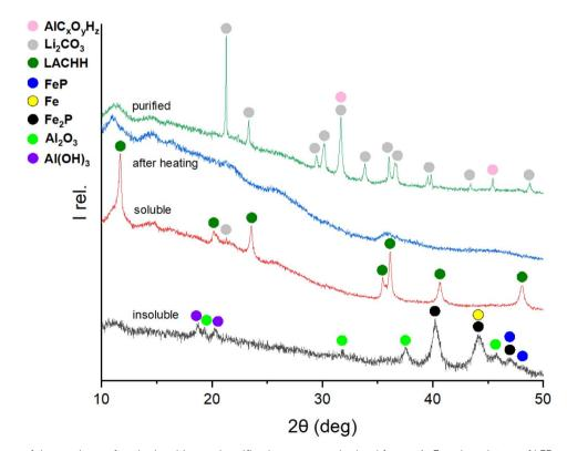
Fig. 6 XRD patterns of the products after the leaching and purification process obtained from a 1:3 molar mixture of LFP and Al ball-milled for 3 h. The most intense Bragg-reflections are assigned to different phases for analysis.
