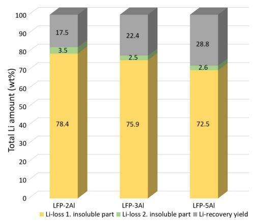
Fig. 7 Comparison of Li-loss during the leaching process and Li-yield of purified Li<sub>2</sub>CO<sub>3</sub> for 1:2, 1:3 and 1:5 molar mixtures of LFP and Al. Liloss was calculated using ICP-OES as explained in the ESI† and lithium recovery yield was calculated by weighing initial mixture and final product. Because of two different methods applied, the total number can exceed 100%.
