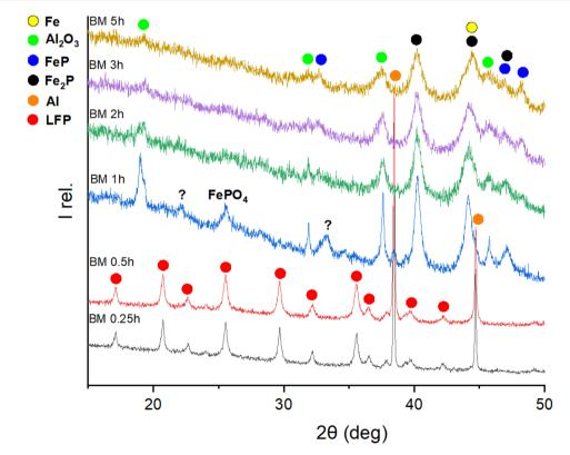
Fig. 2 XRD patterns of a 1:3 molar mixture of LFP and Al measured after different ball-milling times. The most intense Bragg-reflections are assigned to different phases for analysis. The reflections labeled with a question mark cannot be identified because the intensities are too low for a reasonable assignment to a matching phase. 2–3 h are necessary to finish the reaction.
