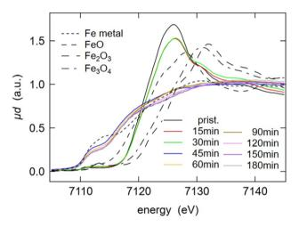
Fig. 4 Fe K-edge X-ray absorption near edge structure (XANES) spectra of pristine LFP and LFP ball-milled with Al metal foil for 0.25 h to 5 h (1:3 molar ratio of LFP to Al). The spectra of iron metal, FeO,  $Fe_2O_3$  and  $Fe_3O_4$  were plotted for comparison.
