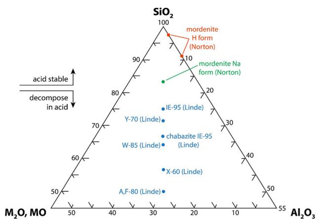
**Fig. 11**  $\text{SiO}_2\text{-Al}_2\text{O}_3\text{-M}_x\text{O}$  ( $\text{M}$  = alkali or alkaline earth,  $x = 1$  or  $2$ ) ternary diagram for zeolite minerals that shows the acid stability<sup>8</sup> (this drawing was modified from ORNL drawing 78-15097<sup>152</sup>).
