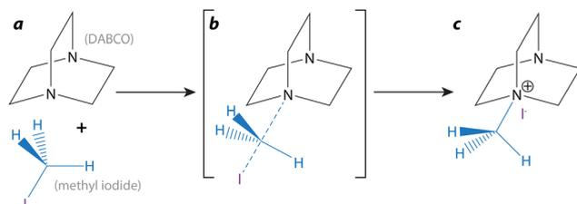
**Fig. 13** The reaction of CH<sub>3</sub>I with DABCO showing (a) the initial forms of each, (b) the intermediate bonding environment, and (c) the final form.<sup>176</sup> This figure was reprinted with permission from Aneheim *et al.*<sup>176</sup> Copyright 2018 Elsevier.
