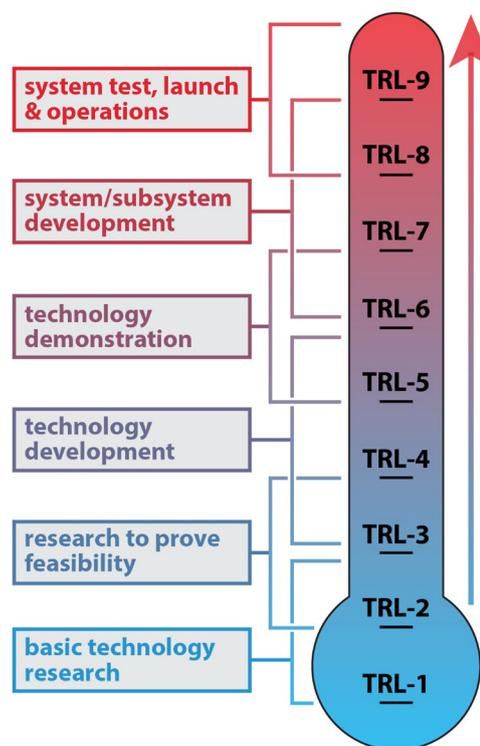
Fig. 5 Technology readiness level (TRL) diagram.<sup>112,113</sup>
