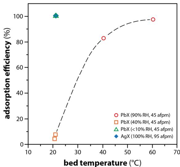
Fig. 4 Comparison of  $I_{2(g)}$  adsorption efficiency as a function of temperature for PbX and Ag. AFPM refers to actual feet per minute (face velocity). This graphic was modified from the original by Maeck and Pence<sup>16</sup> and Staples *et al.*<sup>106</sup>
