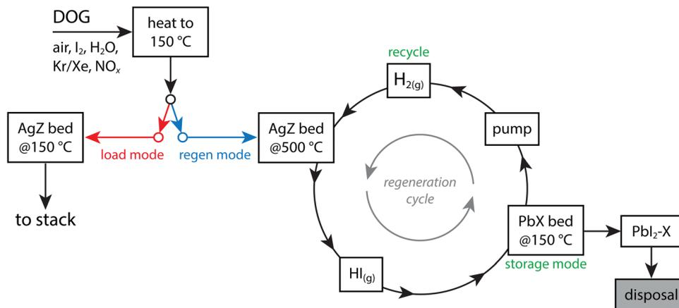
Fig. 3 Process flow diagram showing an AgZ + PbX from Thomas *et al.*<sup>19</sup> showing how the process has an  $I_{2(g)}$  load mode and a regeneration mode where the iodine-loaded AgZ bed is heated under an  $H_{2(g)}$  purge.  $HI_{(g)}$  comes off and reacts with a PbX bed to form  $PbI_2$  [see eqn (4)] for disposal, and recycling the regenerated AgZ bed. This drawing was modified from the original by Thomas *et al.*<sup>19</sup>
