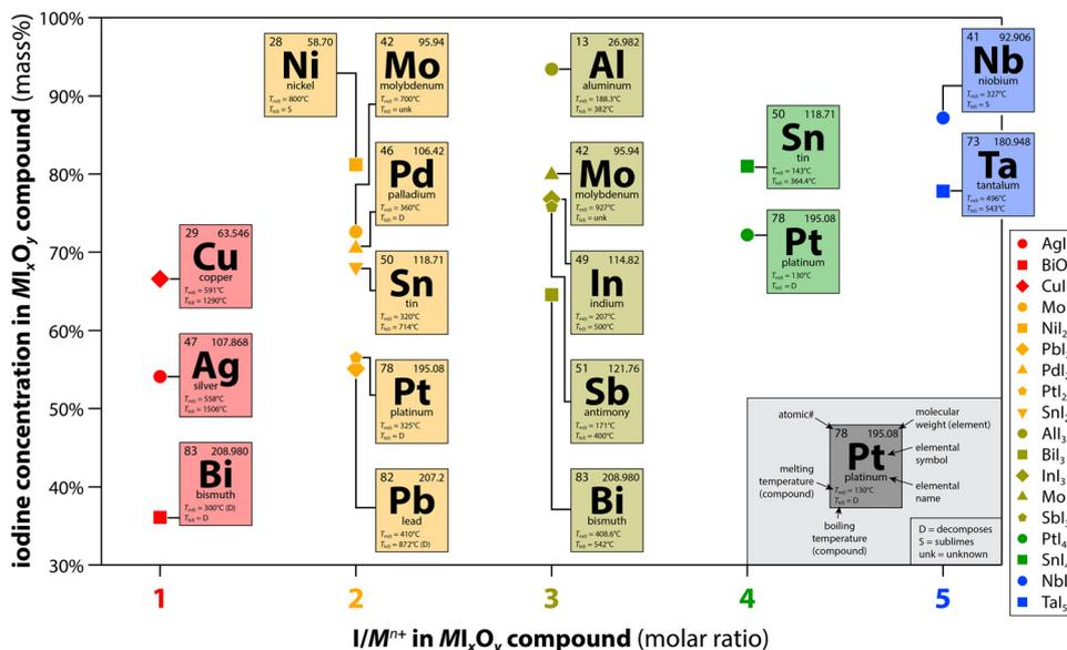
Fig. 7 Summary of the iodine concentration (mass%) for different  $MI_xO_y$  compounds evaluated in the literature. This figure was modified from the original by Riley and Carlson<sup>71</sup> and reprinted with permission. Copyright 2022 Frontiers.
