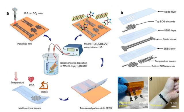
Fig. 6 A wearable multifunctional sensor has been developed with an MXene and graphene composite for health monitoring. (a) Fabrication of the sensor. (b) Various parts of the sensor, (c)  $\varepsilon$  (d) The fabricated sensor on the hand. Reproduced with permission.<sup>58</sup> Copyright 2022 Springer Nature.
