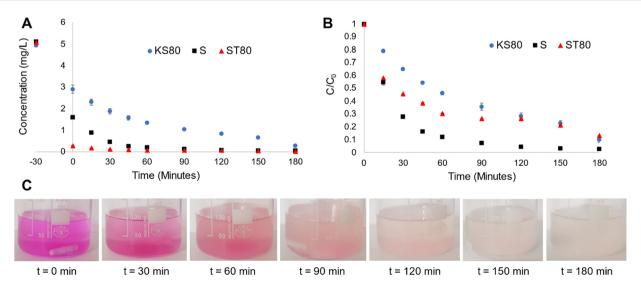
Fig. 6 Rh B degradation study using titanosilicates KS80, S and ST80. (A) Rh B concentration vs. time plots, (B) normalized results  $C/C_0$  vs. time (i.e., final/initial Rh B concentration). (C) Images of Rh B degradation taken throughout the reaction, using sample ST80 as catalyst.
