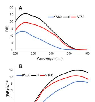
Fig. 3 Diffuse reflectance UV-Vis analysis of titanosilicate samples KS80, S and ST80. (A) Kubelka-Munk plots, (B) Tauc plots
