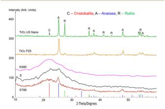
Fig. 4 pXRD patterns for TiO<sub>2</sub> samples US Nano (anatase: rutile 4:1) and Aeroxide P25; and titanosilicate samples KS80, S, ST80. All titanosilicate samples appear to be principally amorphous, in contrast to Aeroxide P25 and US Nano TiO<sub>2</sub> samples
