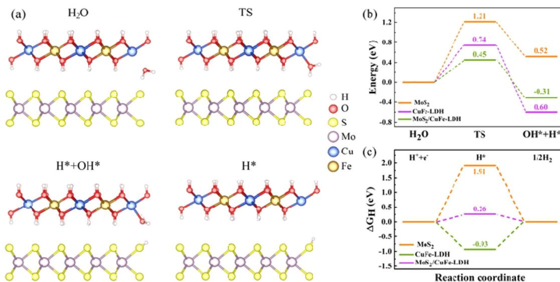
Fig. 7 (a) Optimized structural configurations of the water dissociation process on the CuFe-LDH/MoS<sub>2</sub> heterostructure, (b) computed reaction energy diagram of H<sub>2</sub>O splitting on MoS<sub>2</sub>, CuFe-LDH and the CuFe-LDH/MoS<sub>2</sub> complex, and (c) the associated free energy diagram of hydrogen evolution.
