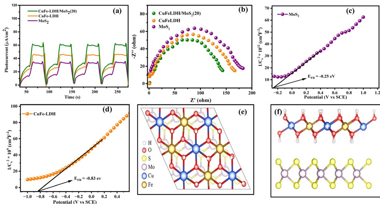
Fig. 6 (a) Response of transient photocurrent, (b) electrochemical impedance spectra of MoS<sub>2</sub>, CuFe-LDH, and CuFe-LDH/MoS<sub>2</sub>(20), (c), (d) Mott-Schottky plots of MoS<sub>2</sub> and CuFe-LDH, (e) top view and (f) side view of the CuFe-LDH/MoS<sub>2</sub> heterostructure.
