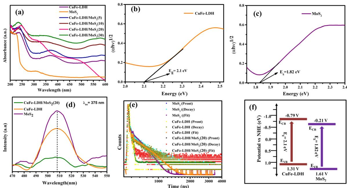
Fig. 3 (a) UV-vis DR spectral graph of the prepared samples and band gap energy values estimated through the Tauc plot of (b) CuFe-LDH, (c) MoS<sub>2</sub>, (d) PL spectra, (e) TCSPS analysis of the MoS<sub>2</sub>, CuFe-LDH, and CuFe-LDH/MoS<sub>2</sub>(20) composites and (f) obtained band gap patterns of the materials.
