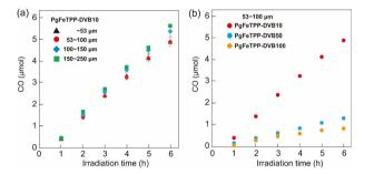
Fig. 8 (a) Photocatalytic activity of PgFeTPP-DVB10 in each classified particle sizes. Black triangles ( $\sim\!53~\mu m$ ), red circles (53–100  $\mu m$ ), blue diamonds (100–150  $\mu m$ ), and green squares (150–250  $\mu m$ ) represent the particle sizes. (b) Photocatalytic activity of PgFeTPP-DVB10 with different cross-linking ratio. DVB feed ratios to total monomer amount are 10 (red circles), 50 (blue circles), and 100 wt% (orange circles), respectively.
