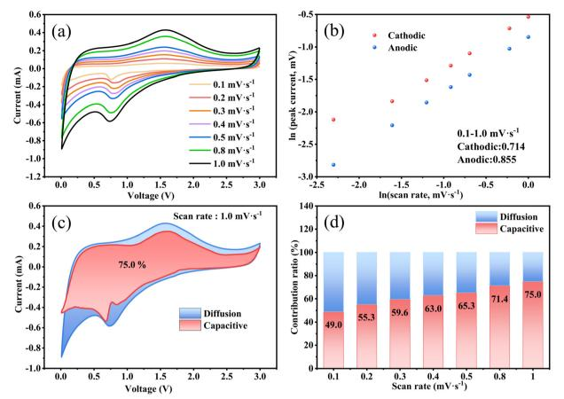
Fig. 5 CV curves of the Fe<sub>7</sub>O<sub>4</sub> QDs@C/RGO composite electrode from 0.1 to 1.0 mV s<sup>-1</sup> (a), the ln(i)-ln(v) plot (b), the capacitive contribution of the  $Fe_3O_4$  QDs@C/RGO composite electrode at 1 mV s<sup>-1</sup> (c) and the pseudocapacitive contribution ratios at different scanning rates (d).
