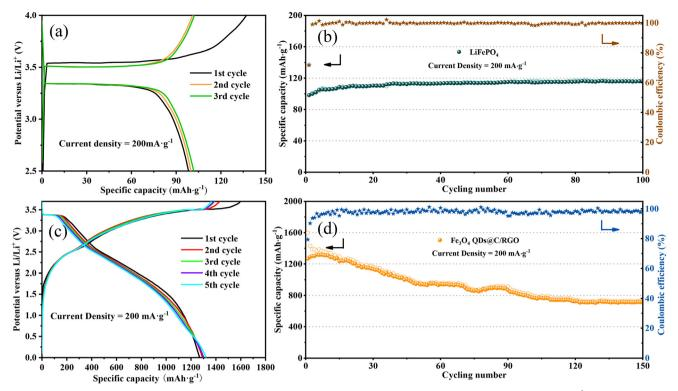
Fig. 8 Charge and discharge voltage profile (a) and cycling performance (b) of a commercial LiFePO<sub>4</sub> cathode at 200 mA g<sup>-1</sup> in half cells. Charge and discharge voltage profile (c) and cycling performance (d) of the Fe<sub>3</sub>O<sub>4</sub> QDs@C/RGO sample in Fe<sub>3</sub>O<sub>4</sub> QDs@C/RGO//LiFePO<sub>4</sub> full cells at 200  $mA q^{-1}$ .
