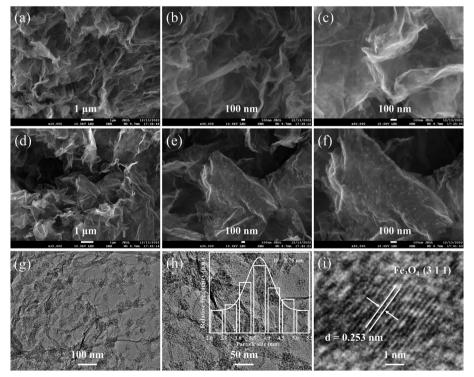
Fig. 3 FESEM images of Fe-BTC/TP-RGO (a-c) and Fe<sub>3</sub>O<sub>4</sub> QDs@C/RGO (d-f) samples under various magnifications. TEM images (g and h) of the Fe<sub>3</sub>O<sub>4</sub> QDs@C/RGO sample under different magnifications with inset showing Fe<sub>3</sub>O<sub>4</sub> particle size distribution. HRTEM image (i) for an individual Fe<sub>3</sub>O<sub>4</sub> nanoparticle in the Fe<sub>3</sub>O<sub>4</sub> QDs@C/RGO sample.
