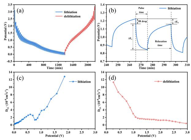
Fig. 6 GITT curves (a) and a profile for a single GITT test (b), and variation of the  $D_{\text{Li}^+}$  values during lithiation (c) and delithiation (d) processes of the Fe<sub>3</sub>O<sub>4</sub> QDs@C/RGO electrode.
