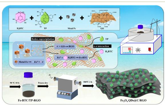
Scheme 1 Schematic illustration for the synthesis of the Fe<sub>3</sub>O<sub>4</sub> QDs@C/RGO sample.
