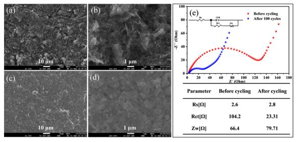
Fig. 7 FESEM images of the  $Fe_3O_4$  QDs@C/RGO electrode before cycling (a and b) and after 100 cycles (c and d) under various magnifications. Nyquist plots of the  $Fe_3O_4$  QDs@C/RGO electrode before cycling and after 100 cycles with inset showing equivalent circuit and the corresponding fitted values of the parameters (e).
