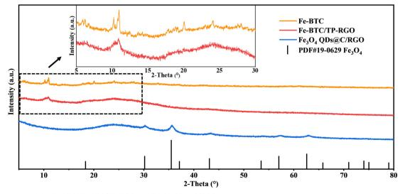
Fig. 1 XRD patterns of the Fe-BTC, Fe-BTC/TP-RGO and Fe<sub>3</sub>O<sub>4</sub> QDs@C/RGO samples
