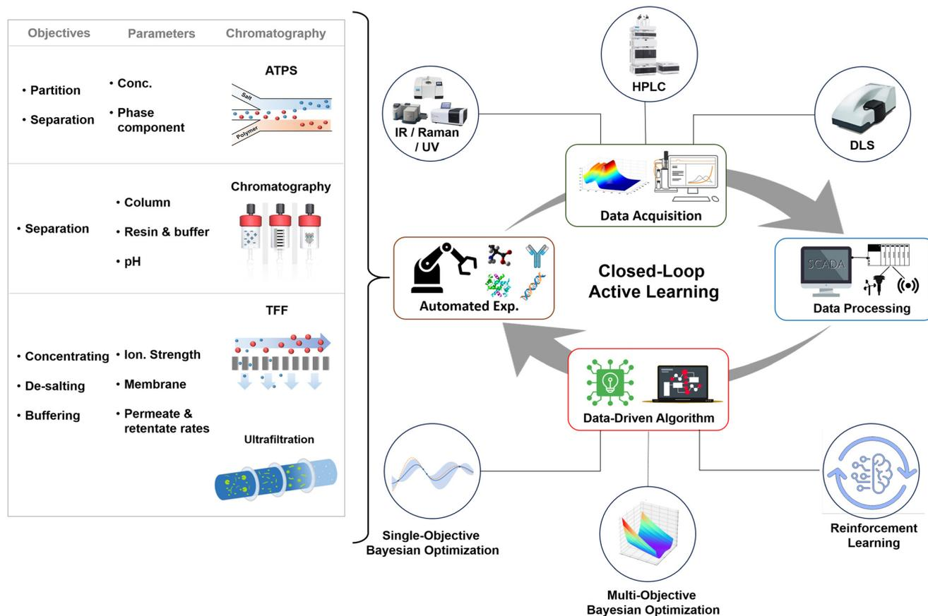
**Fig. 6** Schematic representation of a closed-loop active learning process for a self-driving downstream processing platform illustrating the continuous cycle of automated experimentation, data acquisition, data processing, and decision-making by an AI algorithm, highlighting the autonomous nature of the platform.
