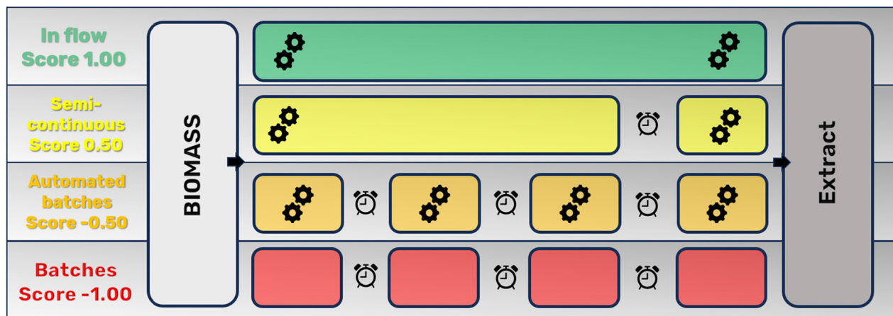
Fig. 5 Scoring based on the scaling options. The gears represent automated systems, and the clocks the time requested between the approaches.
