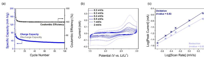
Fig. 4 Performance of SqTI-H composite electrodes in 1 M LiTFSI/1 : 1 DOL + DME, showing (a) cycling performance and coulombic efficiency, (b) scan rate dependence CV, as well as (c)  $\log[\text{scan rate}] - \log[\text{peak current}]$  plot of data from (b) to extract  $b$ -values.
