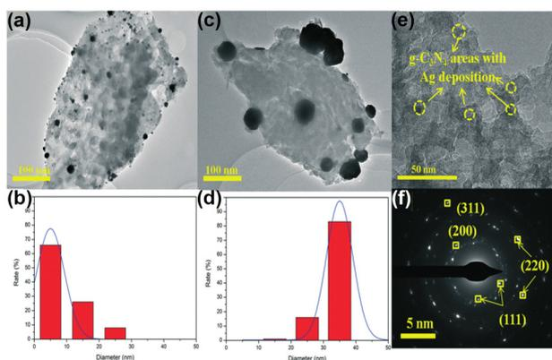
Fig. 14 TEM images (a and c) and Ag nanoparticle size distribution (b and d) of Ag4%/CN (–60) and Ag4%/CN (room) and (e) HR-TEM and (f) SAED of Ag4%/CN (–60). Reprinted with permission from ref. 150. Copyright the Royal Society of Chemistry 2020.
