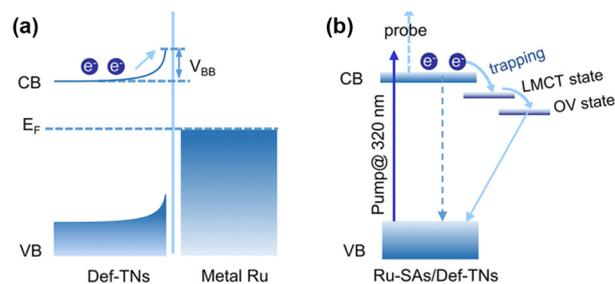
**Fig. 5** Mechanisms underlying the photoexcited electron dynamics involved in (a) Ru-NPs/Def-TNs and (b) Ru-SAs/Def-TNs. Reprinted with permission from ref. 83. Copyright 2020 American Chemical Society.
