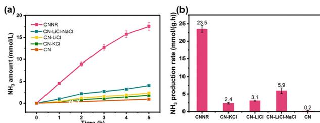
Fig. 13 (a)  $\text{NH}_3$  production from  $\text{N}_2$  reduction with light irradiation time. (b) Photocatalytic  $\text{NH}_3$  production with different  $g\text{-C}_3\text{N}_4$  samples. Reprinted with permission from ref. 144. Copyright 2022 Elsevier B.V.
