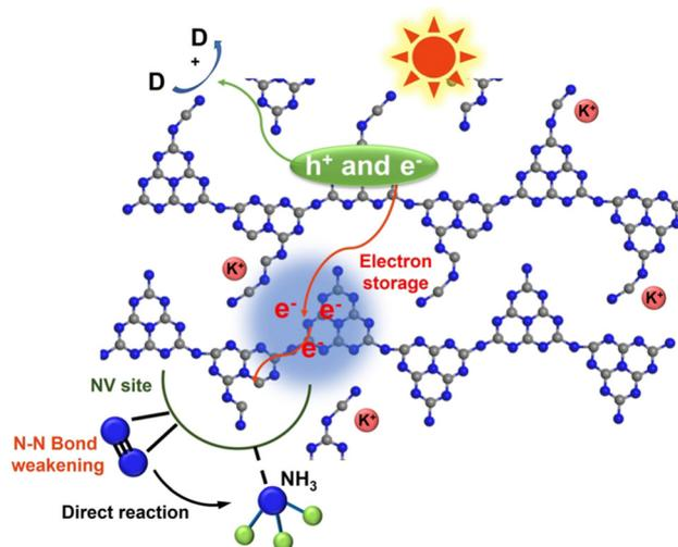
Fig. 12 Schematic diagram of the N<sub>2</sub> reduction reaction over KCCN-NVs. Reprinted with permission from ref. 143. Copyright 2021 Elsevier B.V.
