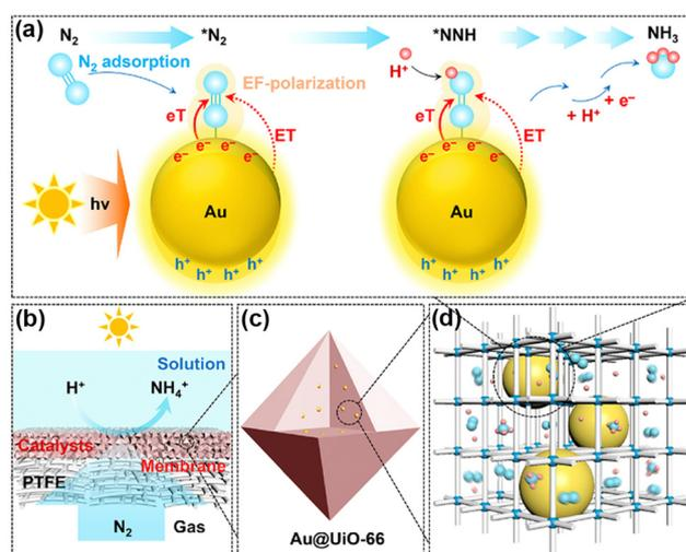
**Fig. 10** Schematic illustration for direct PNRR on Au@UiO-66. (a) Illustration of the direct PNRR on AuNPs. (b) Schematic of the GMS reaction interface design. (c) and (d) Schematic diagram showing the dispersion of plasmonic AuNPs within the cavities of the MOF matrix. Reprinted with permission from ref. 127. Copyright 2021 American Chemical Society.
