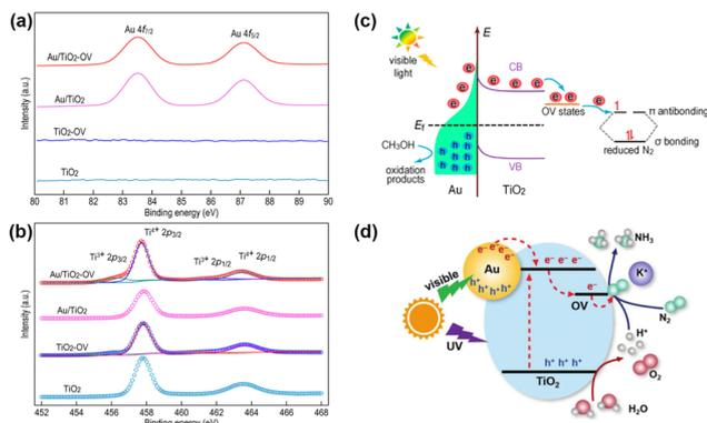
**Fig. 3** (a) and (b) Au 4f and Ti 2p High-resolution XPS spectra of Au/TiO<sub>2</sub>-OV. (c) Schematic illustration of the PNRR process involving plasma hot electrons in Au/TiO<sub>2</sub>-OV. Reprinted with permission from ref. 75. Copyright 2018 American Chemical Society. (d) Schematic diagram of the Au/P25-K<sup>+</sup> PNRR mechanism. Reprinted with permission from ref. 76. Copyright the Royal Society of Chemistry 2019.
