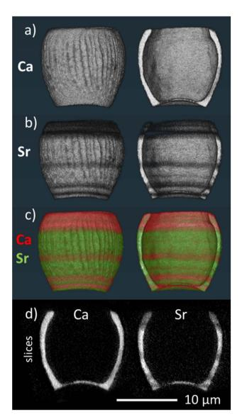
Fig. 2 3D volume renderings of the reconstructed 3D XRF data for (a) calcium and (b) strontium signals individually and (c) combined (calcium signal in red, strontium signal in green), showing both the full image of the lopadolith and a cut through along the growth direction. The corresponding reconstruction slices are also shown (d). For additional views and a blue-yellow rendering, refer to Fig. S3 and S4.† An example XRF spectrum from a single pixel is shown in Fig. S5.†
