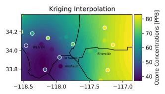
Fig. 5 Hourly ozone heatmap (16:00 on June 22, 2020) using ordinary kriging. The dots with white borders are the evaluation sites, and dots without borders are the training sites.
