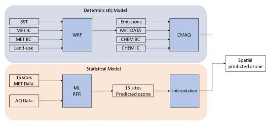
Fig. 4 Flow diagram of the deterministic (CMAQ) and ML models for predicting 2-D ozone concentrations in Southern California, where SST is sea surface temperature, MET IC and MET BC are meteorological initial and boundary conditions, CHEM IC and CHEM BC are chemistry initial and boundary conditions, AQ data is air quality data (NO and NO<sub>2</sub>), and MET data is meteorology data (temperature, relative humidity, wind speed, and wind direction).
