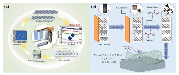
Fig. 15 The combination of acid leaching and thermal treatment for the recycling of spent graphite anode as a closed-loop approach. Reproduced with permission from ref. 138 and 139; Copyright 2023, Elsevier.
