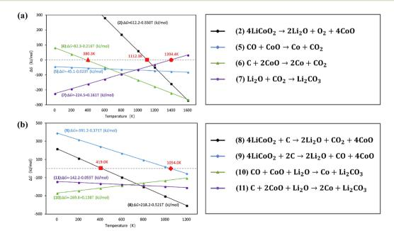
Fig. 9 Thermodynamics analysis of coupling reactions for recycling of cathodes by carbothermic reduction. Reproduced with permission from ref. 102; Copyright 2018, Elsevier.
