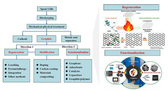
Fig. 7 Schematic illustration of regeneration of functionalization of anodes. Reproduced with permission from ref. 29, 84 and 85; Copyright 2021, American Chemical Society; Copyright 2022, Elsevier; Copyright 2021, Elsevier
