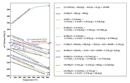
Fig. 11 Thermodynamics analysis for recycling of cathodes with addition of  $NH_4Cl$ . Reproduced with permission from ref. 104; Copyright 2020, American Chemical Society.
