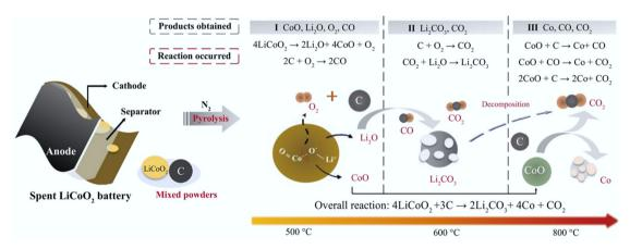
Fig. 5 Schematic illustration of carbothermic reduction during pyrometallurgical processes. Reproduced with permission from ref. 71; Copyright 2020, Elsevier.
