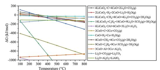
Fig. 10 Thermodynamics analysis for recycling of cathodes with addition of Al foil and pyrolysis gases. Reproduced with permission from ref. 103; Copyright 2022, Elsevier.
