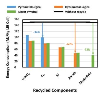
Fig. 21 Reduction in cell production energy by increasing use of recycled materials. Reproduced with permission from ref. 217; Copyright 2018, Elsevier
