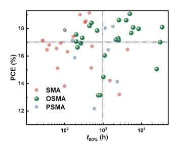
$a_{t_{x_{i_{0}}}}$  indicates the time taken for the PSC performance to degrade to x% of the initial PCE.
