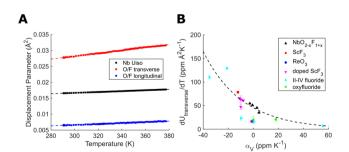
Fig. 3 (A) Refined displacement parameters for NbO<sub>2</sub>F. (B) The gradient of the transverse anion displacement parameter in ReO<sub>3</sub>-type structures showing its relationship with mean volumetric CTE. 14,15,19,25,29-33 Linear fits were performed over the full temperature range of data available for which the structure remains cubic.
