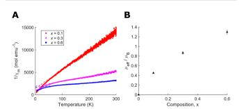
Fig. 4 (A) Inverse magnetic susceptibility against temperature for  $NbO_{2-x}$  $F_{1+x}$  including linear Curie-Weiss fits. Diamagnetic and ferromagnetic corrections have been applied. (B) Effective magnetic moments calculated from Curie-Weiss fitting
