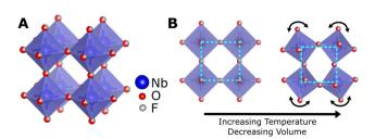
(A) The cubic ReO<sub>3</sub>-type structure of NbO<sub>2</sub>F in the Pm3m space group. (B) An illustration of the rigid unit mode mechanism of negative thermal expansion in the cubic ReO3-type structure.
