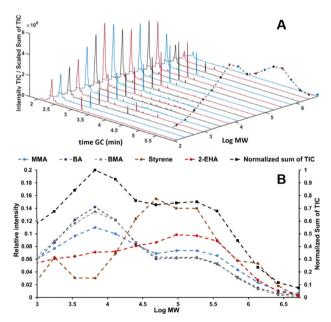
**Fig. 7** SEC-Py-GC-MS results, stacked plot of the obtained Py-GC runs the dashed black line traces the sum of the TIC (A). Relative distribution of monomers over MW of a complex copolymer vs. the chemical composition over the five different monomers present obtained from the Py-GC transformation (B). Adapted from Knol *et al.*, *J. Chromatogr. A*, 2023 under the CC-BY license. 113
