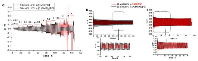
Fig. 6 (a) Rate capability of the 50 mol% LiFSI in [P<sub>1</sub>(DMA)<sub>3</sub>][FSI] and [HMG][FSI] in Li symmetrical cell, 1 hour polarization time at 50 °C, (b) long term cycling of the 50 mol% LiFSI in  $[P_1(DMA)_3][FSI]$  and [HMG][FSI] in Li symmetrical cell at 0.5 mA cm<sup>-2</sup> (c) 1.5 mA cm<sup>-2</sup>, 0.5 mA h cm<sup>-2</sup> at 50 °C.
