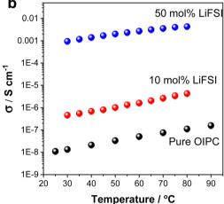
Fig. 2 (a) DSC heating traces (b) ionic conductivity, of the pure OIPC  $([P_1(DMA)_3][FSI])$ , 10 mol% and 50 mol% LiFSI in the OIPC.
