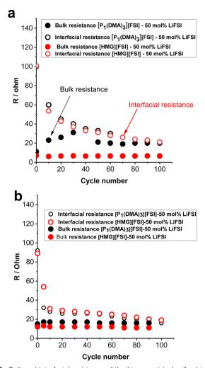
Fig. 7 Bulk and interfacial resistance of the Li symmetrical cells obtained before polarisation and after every 10 cycles for  $[P_1(DMA)_3][FSI]-50$  mol% LiFSI and [HMG][FSI]-50 mol% LiFSI, (a) 0.5 mA cm $^{-2}$  (0.5 mA h cm $^{-2}$ ), (b) 1.5 mA cm $^{-2}$  (0.5 mA h cm $^{-2}$ ).
