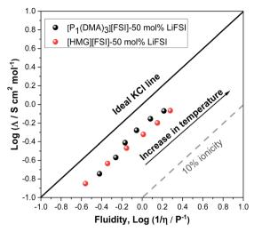
Fig. 5 Walden plot showing relationship between inverse viscosity and molar conductivity for 50 mol% LiFSI in [P<sub>1</sub>(DMA)<sub>3</sub>][FSI] and 50 mol% LiFSI
