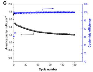
Fig. 9 (a) Rate capability of Li|50 mol% LiFSI/[ $P_1(DMA)_3$ ][FSI]|LFP (b) Cycling performance of Li|50 mol% LiFSI/[ $P_1(DMA)_3$ ][FSI]|LFP and Li|50 mol% LiFSI/[HMG][FSI]|LFP at C/5 and (c) Cycling performance of Li|50 mol% LiFSI/[ $P_1(DMA)_3$ ][FSI]|LFP at C/2 rate at 50°.
