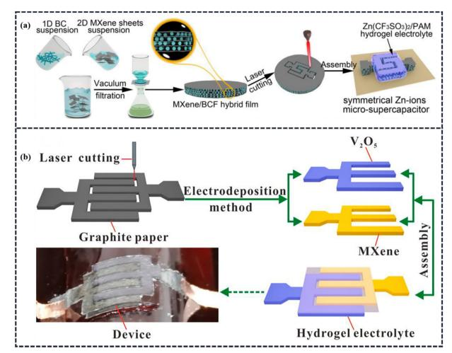
Fig. 14 (a) Illustration of the complete fabrication process of the symmetrical agueous Zn-ion-based MSCs with MXene/BCF hybrid film electrodes. (Reproduced from ref. 122 with permission from Elsevier). (b) The preparation and assembly process of the ZIMSC based on the Ti<sub>3</sub>C<sub>2</sub>T<sub>x</sub> MXene anode, V<sub>2</sub>O<sub>5</sub> cathode, and ZnSO<sub>4</sub>/PAM hydrogel electrolyte. (Reproduced from ref. 85 with permission from Elsevier).
