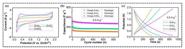
Fig. 10 (a) Comparison of CV curves at a scan rate of 10 mV s<sup>-1</sup> for the TiN electrode tested in different electrolytes including  $Zn(CH_3COO)_2$ ,  $ZnCl_2$ , and  $ZnSO_4$ . (b) cycling performance and (c) corresponding GCD curves of the Zn-TiN capacitor in different electrolyte media. (Reproduced from ref. 89 with permission from Wiley).
