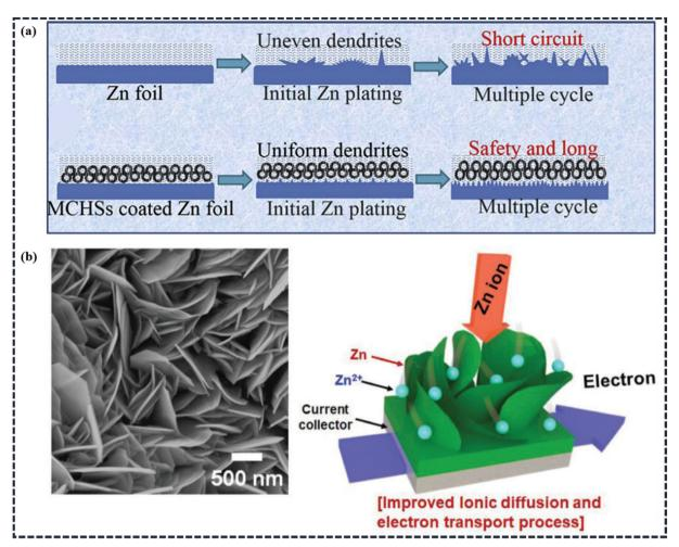
(a) Schematics illustration showing the morphological progression for bare and MCHSs-coated Zn foils during Zn stripping/plating cycling (Reproduced from ref. 45 with permission from Elsevier). (b) FESEM image of 2D Zn, and schematic illustration of the 2D and hierarchically nanostructured Zn (2D-Zn) metal electrode for plating/stripping processes. (Reproduced from ref. 97 with permission from Wiley).
