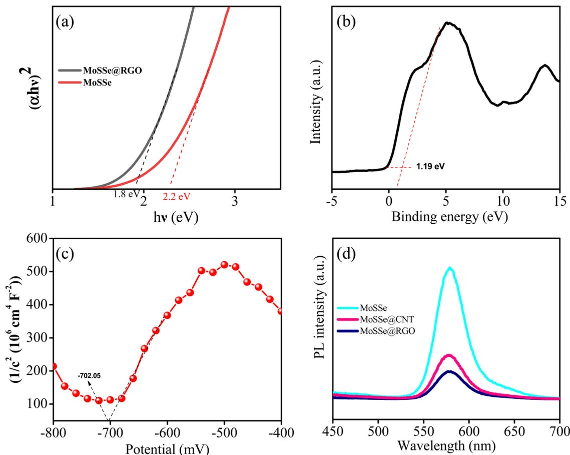
Fig. 7 (a) Tauc plot of MoSSe and the MoSSe@RGO nanocomposite; (b) VB XPS spectra and (c) Mott–Schottky plots of the MoSSe@RGO nanocomposite; (d) PL spectra of an aqueous solution of eosin Y ( $1.0 \times 10^{-7}$  M, excitation wavelength = 490 nm) in the presence of MoSSe@CNT and MoSSe@RGO.
