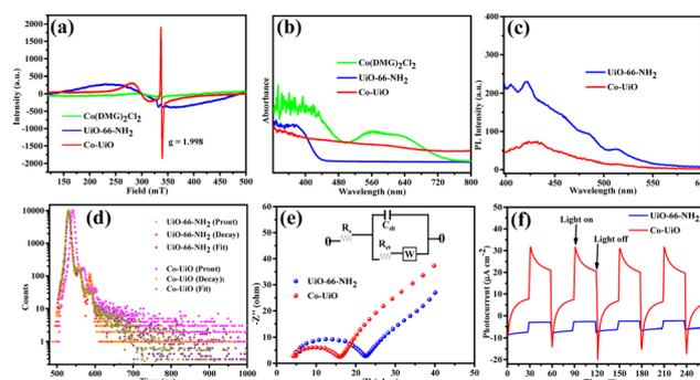
**Fig. 3** (a) EPR spectra, (b) UV-Vis diffuse reflectance spectra, (c) photoluminescence (PL) emission spectra, (d) time-resolved photoluminescence decay profile, (e) EIS Nyquist plots (Inset: The equivalent circuit), and (f) transient photocurrent response of the as-synthesised catalyst.
