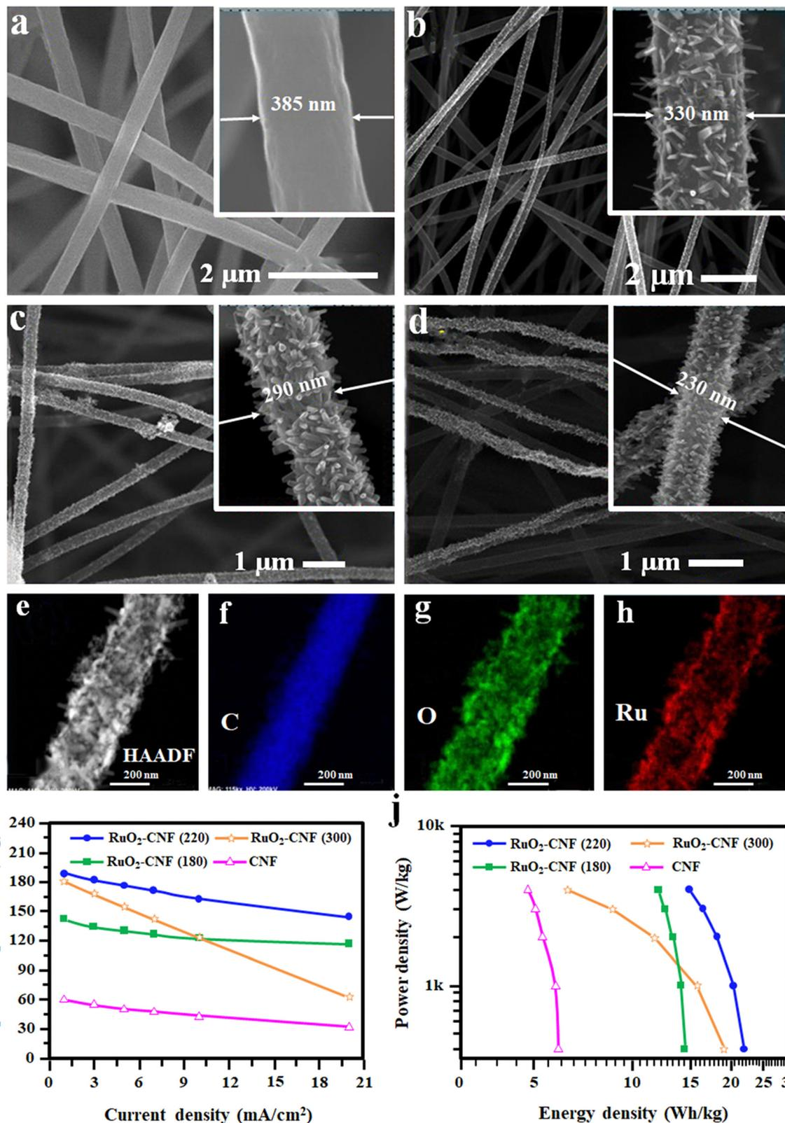
Fig. 10 (a)–(d) FE-SEM images of pure and RuO<sub>2</sub>-doped CNF. (e)–(h) TEM and EDS analysis of RuO<sub>2</sub>-CNF. (i) Specific capacitance with different current densities and (j) Ragone plot of RuO<sub>2</sub>-CNF flexible SC. Reproduced from ref. 102 with permission from American Chemical Society, copyright 2020.
