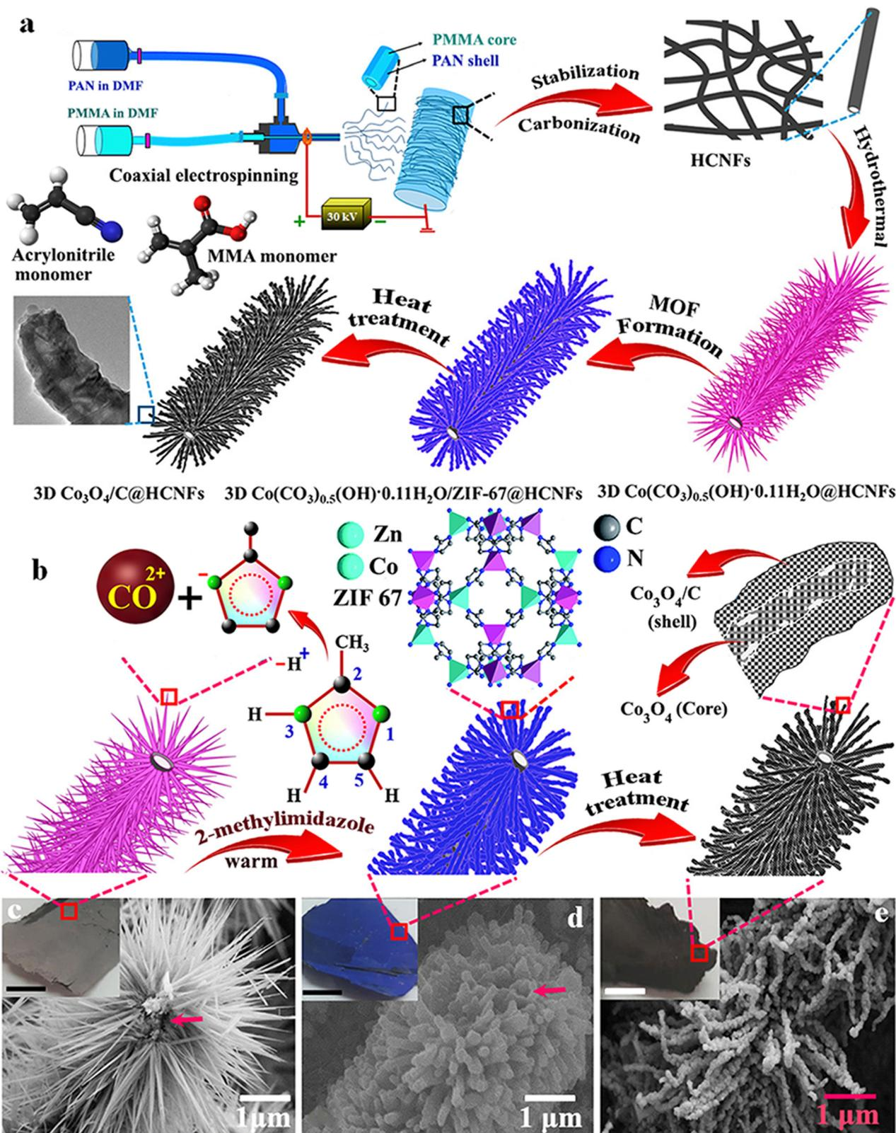
**Fig. 14** (a and b) Schematic and mechanism of the fabrication of  $3\text{D Co}_3\text{O}_4/\text{C@HCNF}$  nanocomposites. FE-SEM image of (c)  $\text{Co}(\text{CO}_3)_{0.5}\text{OH}\cdot 0.11\text{H}_2\text{O@HCNFs}$ , (d)  $\text{Co}(\text{CO}_3)_{0.5}\text{OH}\cdot 0.11\text{H}_2\text{O}/\text{ZIF-67@HCNFs}$  and (e)  $\text{Co}_3\text{O}_4/\text{C@HCNFs}$ . Reproduced from ref. 121 with permission from American Chemical Society, copyright 2020.
