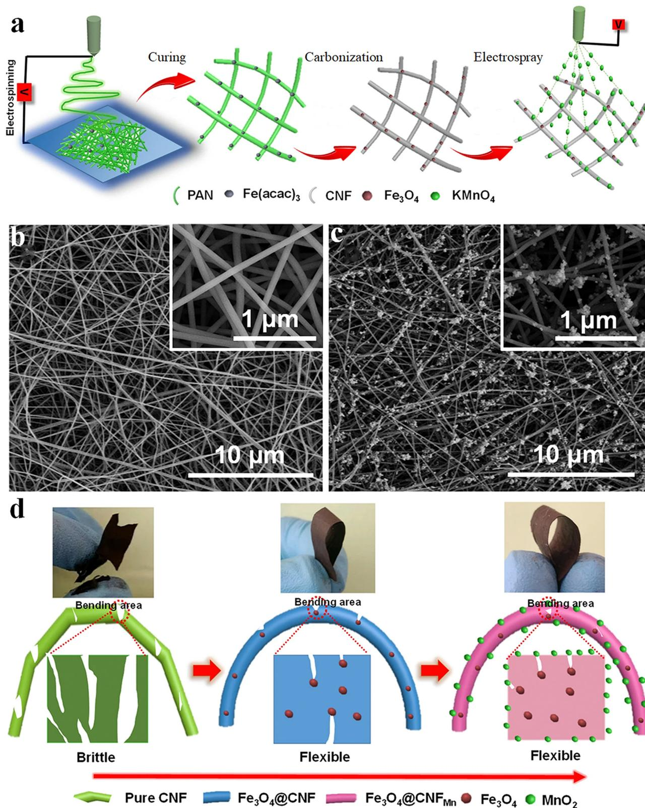
Fig. 12 (a) Schematics of flexible  $\text{Fe}_3\text{O}_4$ @CNFMn electrode preparation. (b and c) FE-SEM micrographs of the  $\text{Fe}_3\text{O}_4$ @CNF and  $\text{Fe}_3\text{O}_4$ @CNFMn fiber electrode respectively. (d) Photographs and mechanism of the enhanced flexibility of the  $\text{Fe}_3\text{O}_4$ @CNFMn electrode. Reproduced from ref. 108 with permission from Nature, copyright 2017.
