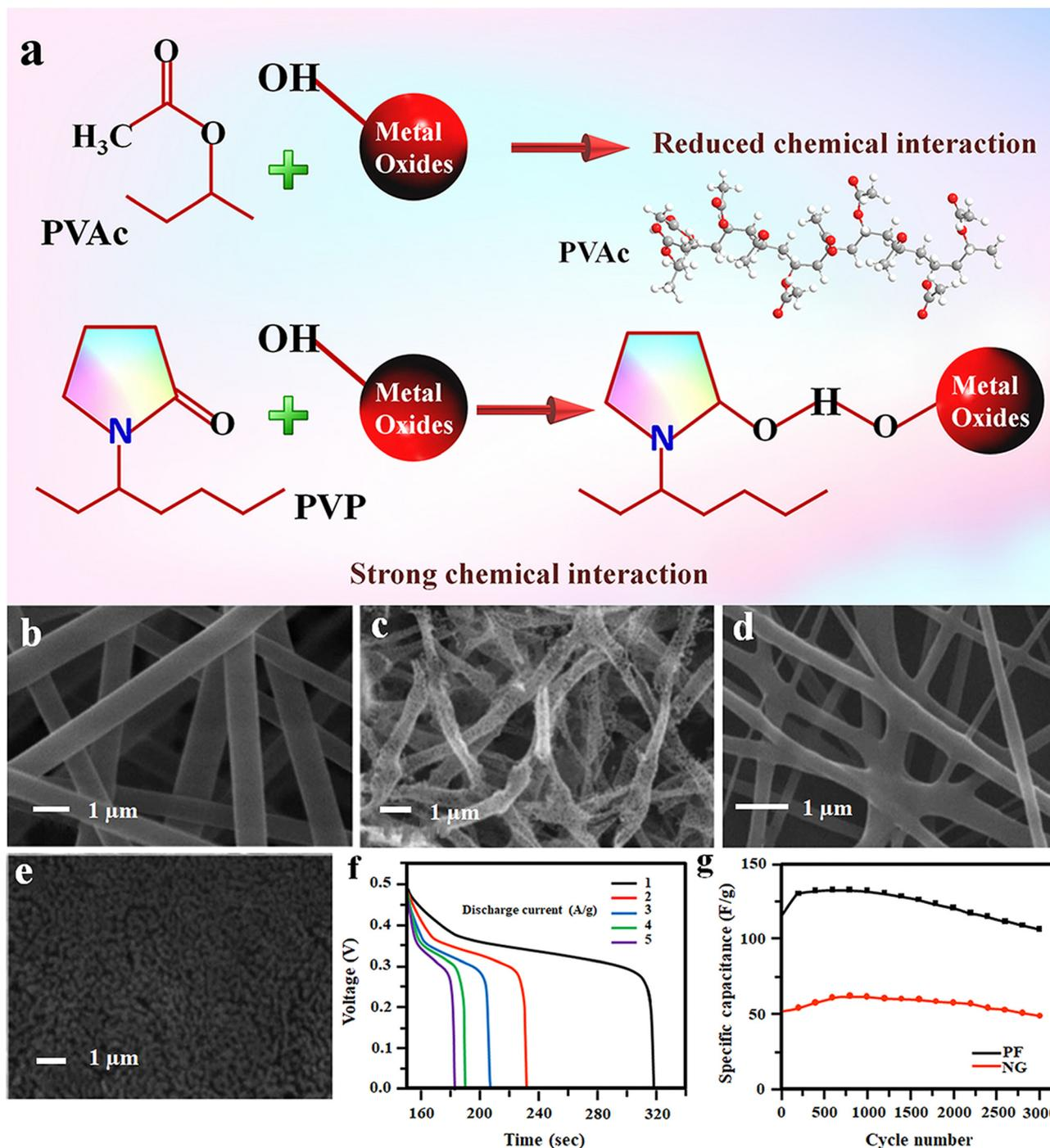
**Fig. 11** (a) Schematic showing the interactions of metal oxides with different polymers (PVAc and PVP). (b)–(e) FE-SEM micrographs of as spun and calcined  $\text{Fe}(\text{acac})_3$ -PVP and  $\text{Fe}(\text{acac})_3$ -PVA electrospun fibers, respectively. (f) Discharge curves of PF at various current densities. (g) Comparison of the cycling performance of both PF and NG electrodes. Reproduced from ref. 103 with permission from Royal Society of Chemistry, copyright 2013.
