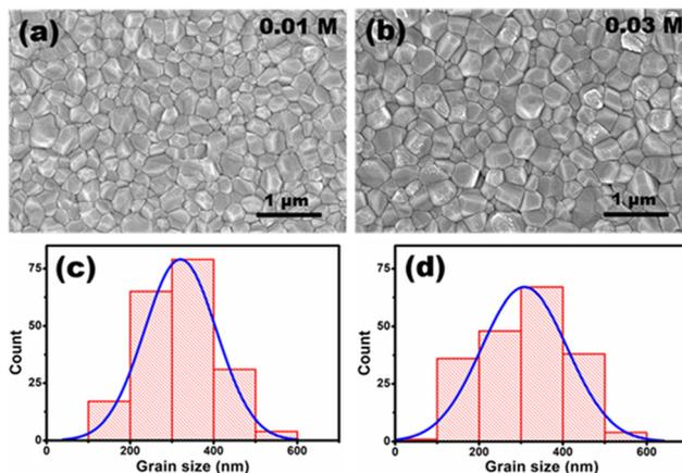
Fig. 4 SEM images of perovskite films deposited on different concentrations of [TMPA][TFSI] ionic liquid-treated TiO<sub>2</sub> compact layers: (a) 0.01 M, and (b) 0.03 M. The corresponding grain size distribution of (c) 0.01 M, and (d) 0.03 M of ionic liquid modification.
