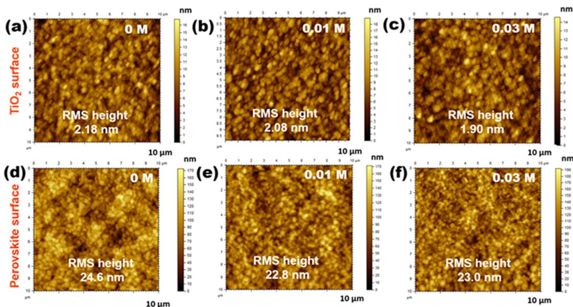
Fig. 3 AFM images of the TiO<sub>2</sub> compact layers coated with different concentrations of [TMPA][TFSI] ionic liquid: (a) 0 M, (b) 0.01 M and (c) 0.03 M. AFM images of the perovskite films grown on [TMPA][TFSI] coated TiO<sub>2</sub> compact layer: (d) 0 M, (e) 0.01 M and (f) 0.03 M.
