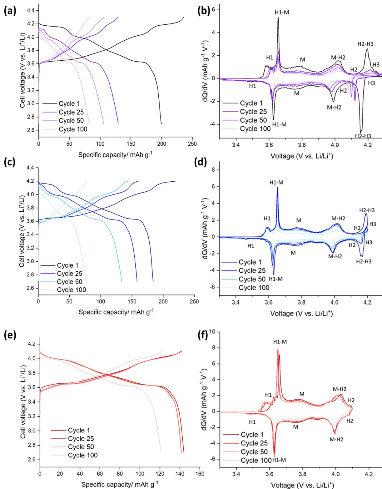
**Fig. 3** Electrochemical performance during galvanostatic charge and discharge of SS-LNO/Li half cells at  $10 \text{ mA g}^{-1}$ : (a) between 2.7–4.3 V (b) corresponding differential capacity ( $dQ/dV$ ) plot with phases (c) between 2.7–4.2 V (d) corresponding differential capacity ( $dQ/dV$ ) plot with phases (e) between 2.7–4.1 V (f) corresponding differential capacity ( $dQ/dV$ ) plot with phases.
