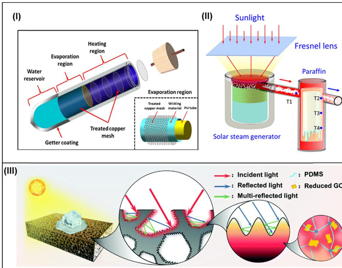
Fig. 14 Other potential applications of SIWE devices. (I) A portable solar steam generator. Reproduced with permission.<sup>179</sup> Copyright 2019, American Chemical Society. (II) Schematic setup for outdoor removal of paraffin deposits on the walls of oil pipelines. Reproduced with permission.<sup>200</sup> Copyright 2019, American Chemical Society. (III) A photothermal active deicing device performance. Reproduced with permission.<sup>201</sup> Copyright 2020, Royal Society of Chemistry.
