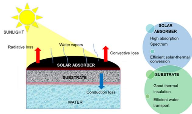
Fig. 1 Schematic illustration of solar-driven interfacial water evaporation.
