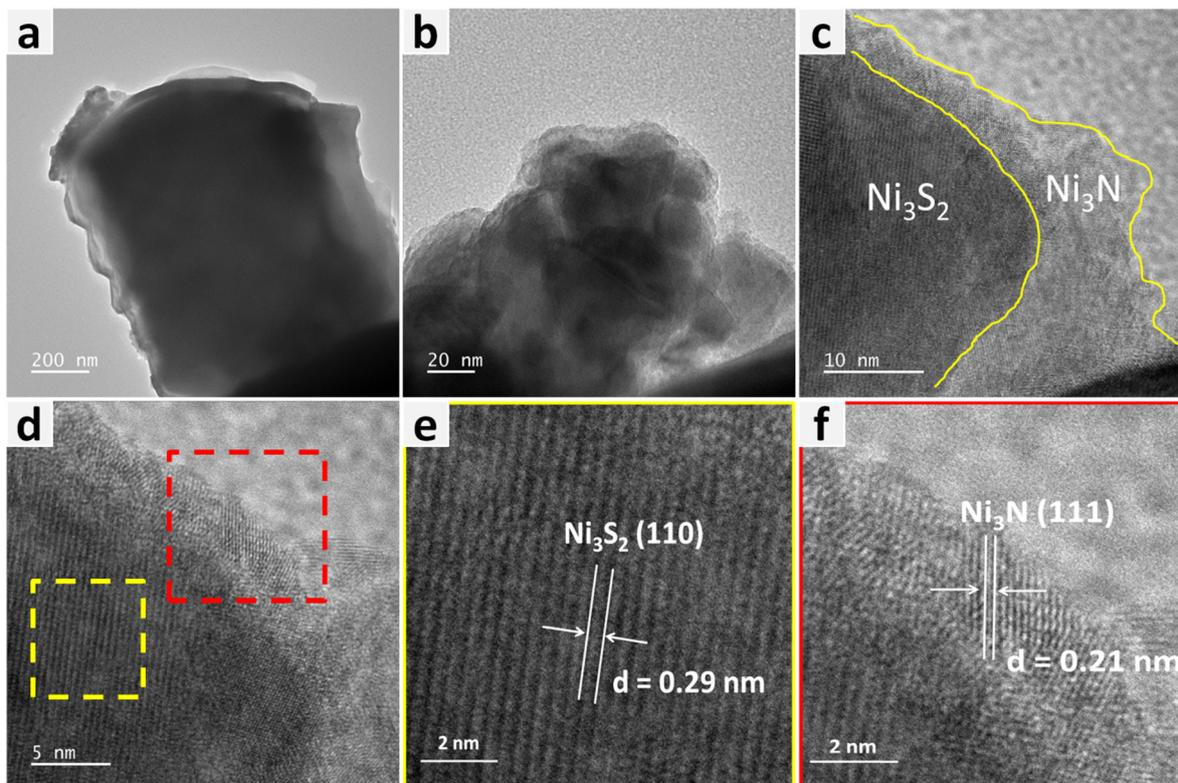
Fig. 3 (a and b) The TEM images of 2-D nanosheets showing the heterostructure of  $\text{Ni}_3\text{S}_2$ - $\text{Ni}_3\text{N}$ . (c and d) The HRTEM images of  $\text{Ni}_3\text{S}_2$ - $\text{Ni}_3\text{N}$  showing the formation of an interface between  $\text{Ni}_3\text{S}_2$  and  $\text{Ni}_3\text{N}$ . (e and f) The HRTEM images showing the presence of  $\text{Ni}_3\text{S}_2$  and  $\text{Ni}_3\text{N}$  phases with the corresponding fringe widths.
